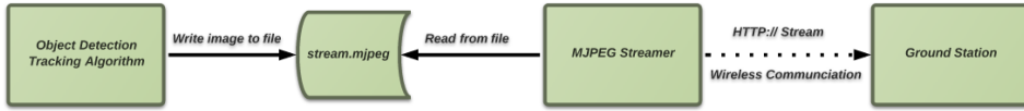
Figure 5.5: The tracking algorithm writes the images that it processes (with marked object locations) to a file stored on the SBC. The video streamer reads from this file, and streams its content over the HTTP protocol. The control station views the stream by connecting to the correct HTTP address.
