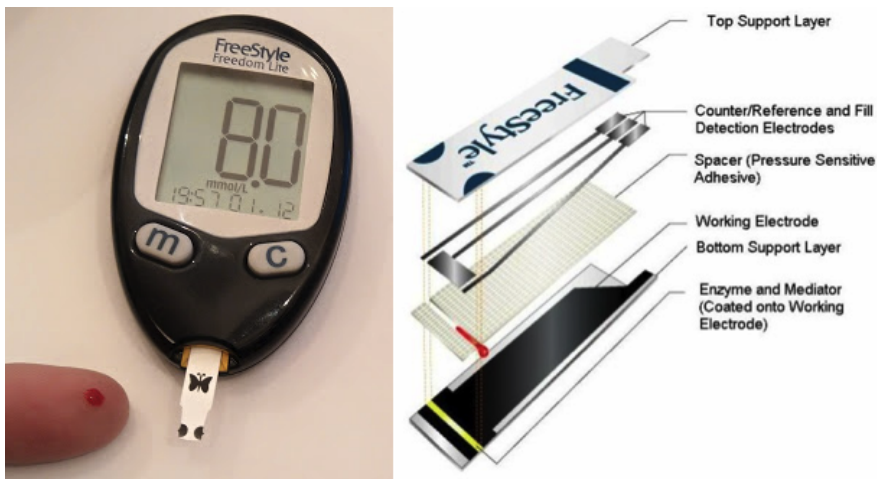
Figure 3.1: SMBG meter. The strip is an electrochemical device that receives a small drop of blood. The blood is transported into the strip by lateral flow, and comes into contact with enzymes inside the strip (hexokinase or glucose oxidase) that generate a current proportional to the glucose concentration in the blood. The current is read by the meter, and converted to a glucose concentration.
