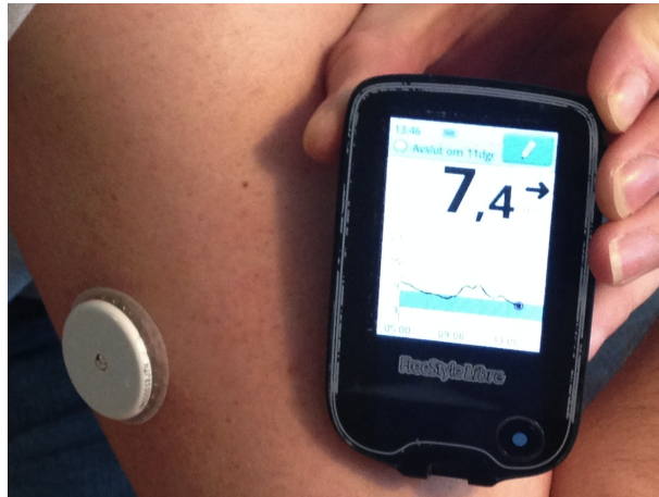
Figure 3.3: The FreeStyle Libre from Abbott. Shown here is the sensor (white) situated on the arm and the receiver (black) used to scan the sensor. The scanning can also be done using a Near Field Communication (NFC) enabled smartphone. Image from creative commons, license: CC BY-SA 4.0
