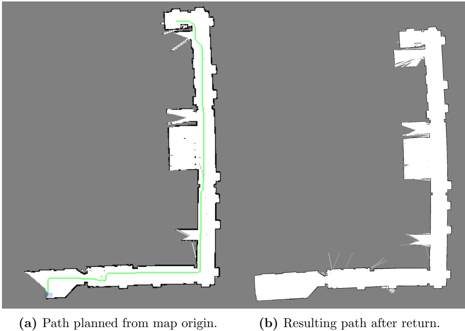
Figure 5.10: Figure 5.10a shows the path planned from the map’s origin to the most remote point of the map before path following began. Figure 5.10b shows the map after the robot successfully traversed the map to the most remote location and back, using path planning and path following both ways. The figure on the left is a screenshot and is thus depicted at a slightly lower resolution.
