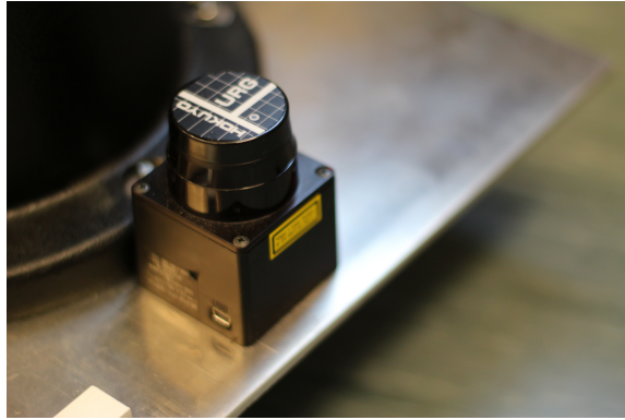
Figure 3.1: The URG-04LX-UG01 LIDAR unit by Hokuyo , an entry level LIDAR recommended for use with autonomous robots by the manufacturer, as mounted on the robot.
