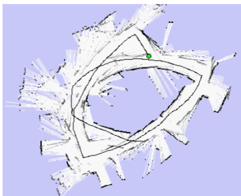
Figure 2.4: Mapping based on raw odometry. The map is highly inconsistent and is hard to interpret. Image courtesy of Sebastian Thrun, robots.stanford.edu , screenshot of video demonstration Raw Data of Intel Research Lab .
