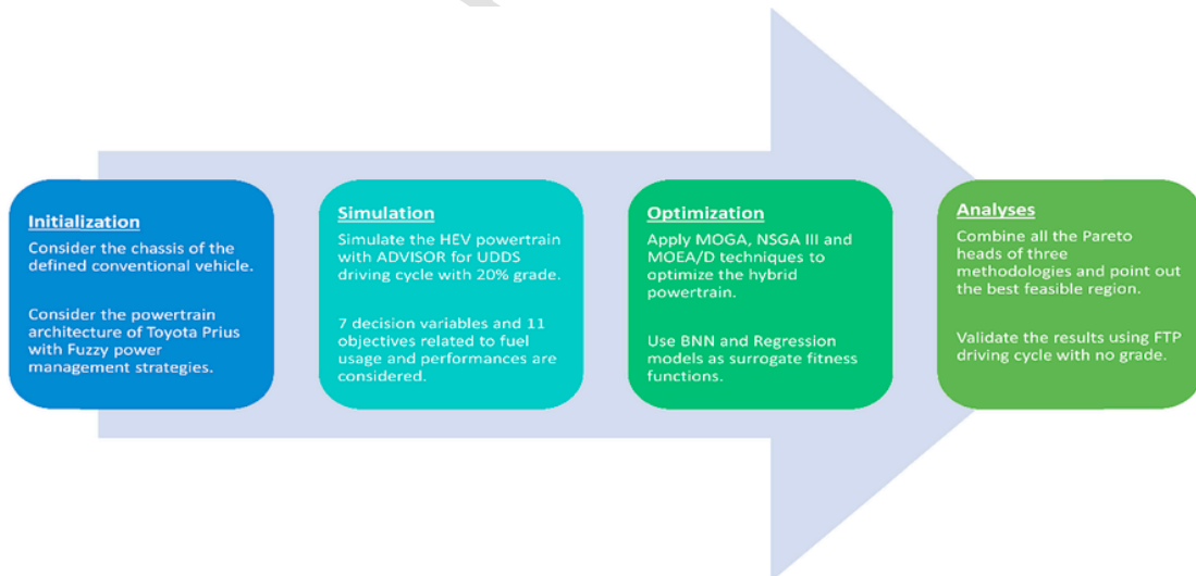
Fig. 1. Proposed work-flow for multi-objective HEV powertrain optimization.
