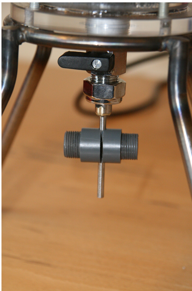
Figure 66: Picture of the magnet holder when mounted on the pipe. Notice the (manual) valve at the outlet of the reservoir.
