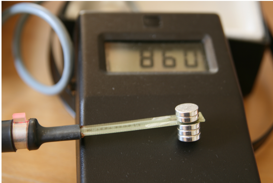
Figure 53: How the magnetic field addition and subtraction tests were performed using the teslameter and the permanent magnets.
