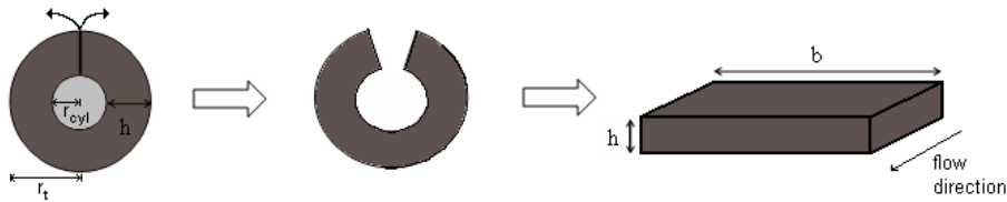
Figure 24: Illustration of the pipe with the cylinder constriction inside, and a comparison with a rectangular flow regime
