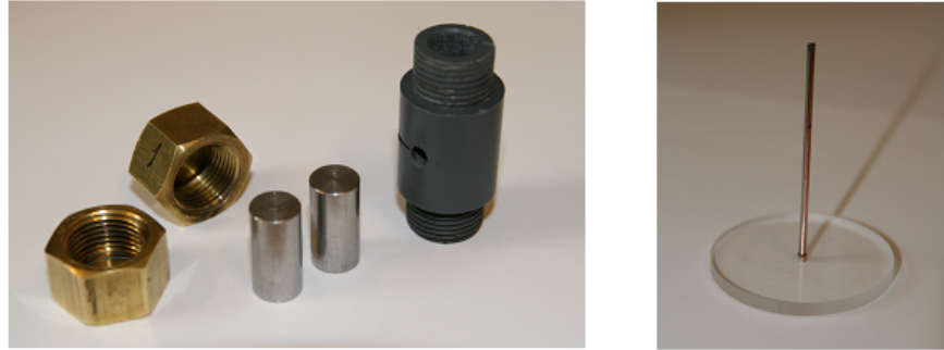
Figure 67: Picture of the magnet holder to the left, with the cap and iron cylinder used to push the magnets, and the cylinder constriction to the right. The constriction is a welding rod mounted on a piece of plexiglass.
