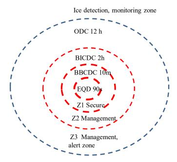
Figure 5. Four IM zone definitions (ISO 35104-2018) for the example Blow Out Preventer (BOP) case indicating required termination time for entering the defined safe states.
