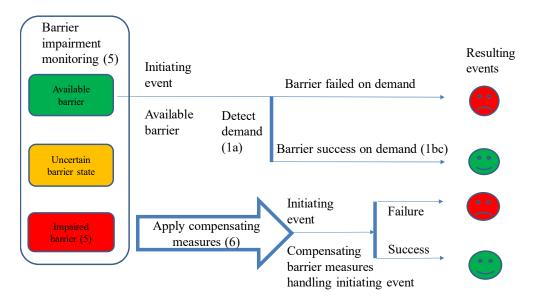
Figure 7. The box to the left indicates operational monitoring barrier states (availability/ impairment). The upper event tree presents the normal barrier events (labc). The blue arrow and lower event tree represents how the operator may decide to apply predefined compensating measures(6) in case of indicated barrier impairment(5).
