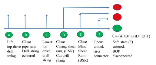
Figure 10. Illustration of detailed BOP actions in an event tree for the operator barrier panel.
