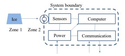
Figure 11. System boundary for an ice detector including subsystems.
