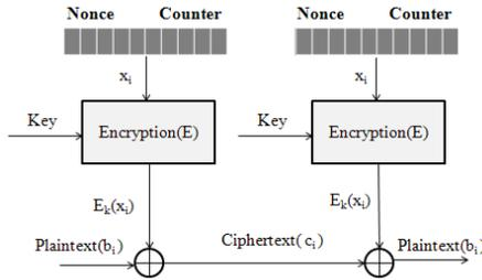
Fig. 2: CTR encryption and decryption process.
