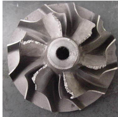
FIGURE 2.2: Damaged impeller, performance turbochargers (2013)
