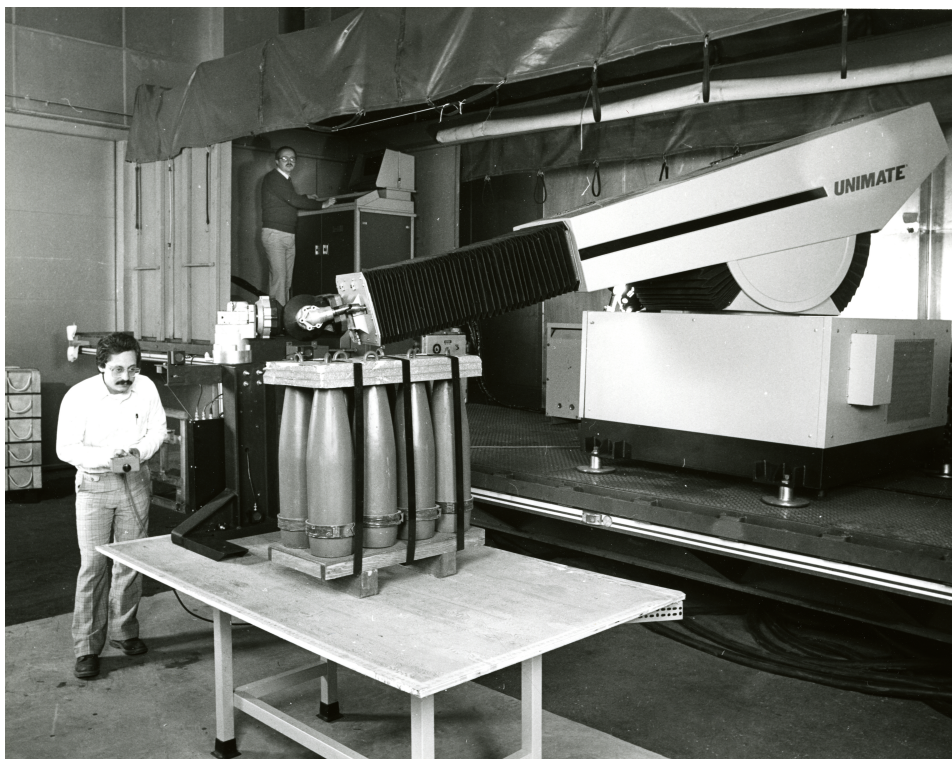
Figure 2.1: A Unimate at the Automated Manufacturing Research Facility (ca. 1983) being taught a new setpoint. Image courtesy of the National Institute of Standards and Technology Digital Collections, Gaithersburg, MD 20899 [21].
