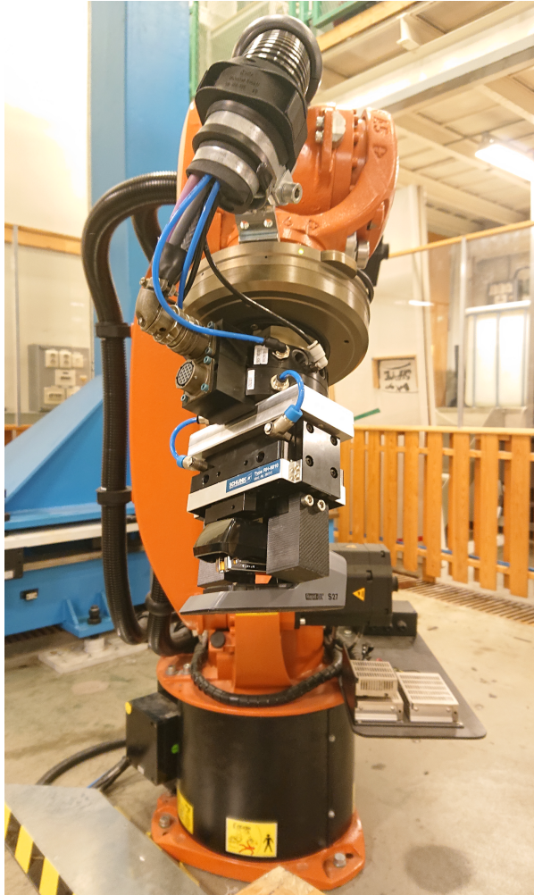
Figure 17: KR 16 ready to transfer the stapler from one location to another using a pneumatic SCHUNK gripper with 3D printed fingers.
