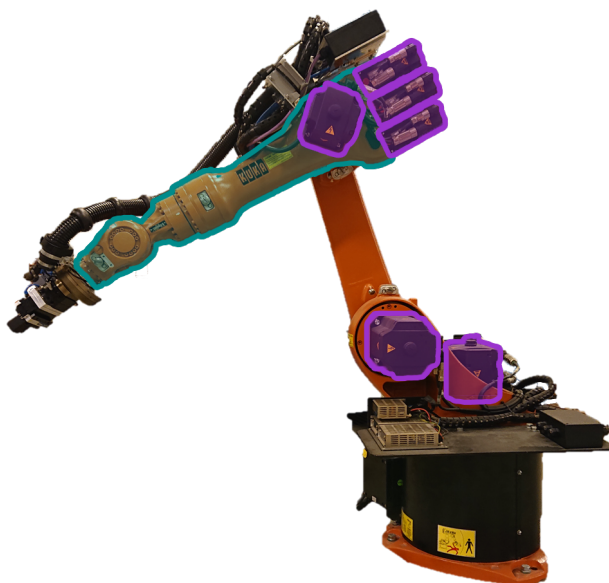
Figure 3.2: The KUKA KR16-2 industrial robot with motors highlighted in purple and the long transmission down link A3 highlighted in green.
