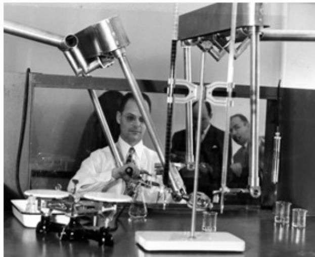
Figure 2.9: Raymond C. Goertz used bilateral teleoperation in early 1950s to handle radioactive material [58].
