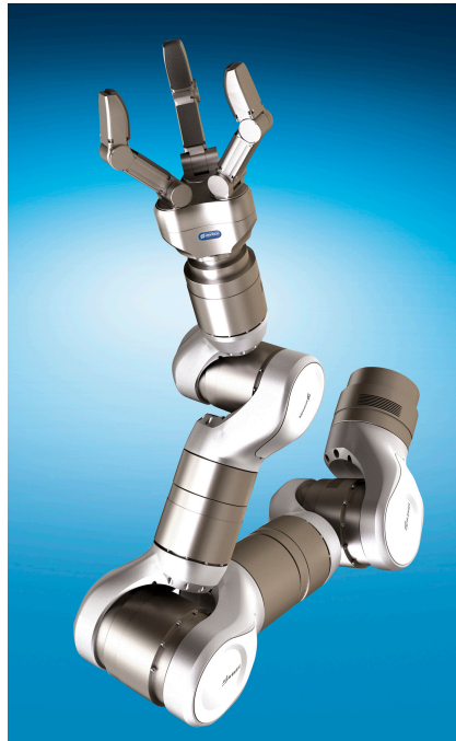
Figure 3.5: LWA3, manipulator from Schunk GmbH & Co. KG, Germany [122].
