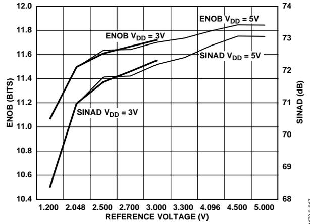
Figure 17. AD7994 SINAD/ENOB vs. Reference Voltage, Mode 1, 121 kSPS
