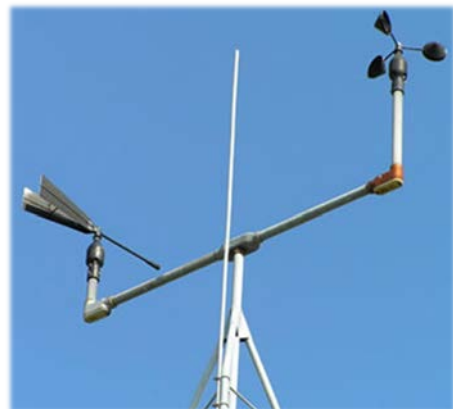
Figure 22. Anemometer and wind vane
