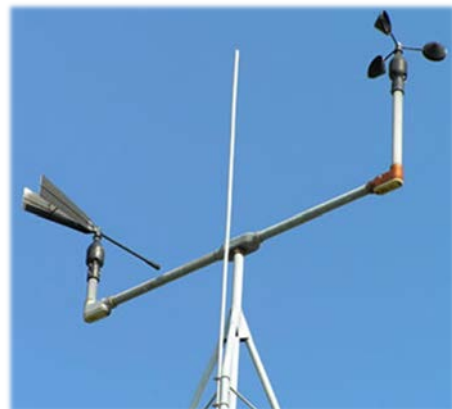
Figure 22. Anemometer and wind vane
