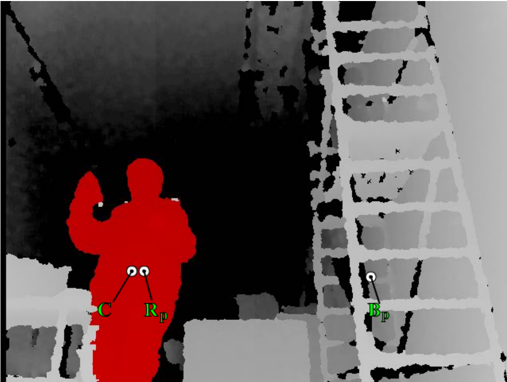
Figure 5.1.: The distance between R_p (Red previous) and C (Current), and the distance between B_p (Blue previous) and C are calculated, and the shortest distance to each “current point” is selected. In the image above, the C had the shortest distance to the red label and therefore it was marked as red.
