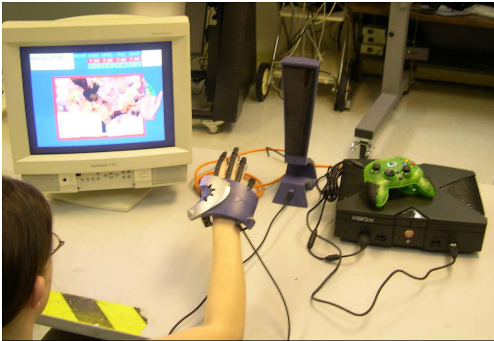
Figure 2.1.: The P5 data glove is a low-cost data glove with a 3D-positioning sensor. Image from [22].
