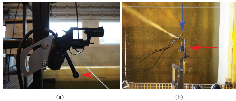
Figure 3.5: (a) Photo of the signalgun and near field hydrophone indicated by red the arrow. (b) Top view of the experimental set up with signalgun (red arrow) and hydrophones (blue arrow).
