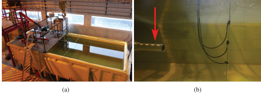
Figure 3.3: (a) Photo of the water tank with dimensions 6 m x 2.5 m x 1.4 m. (b) Underwater photo with gun port of watergun on the left side (red arrow) and hydrophones in the middle.
