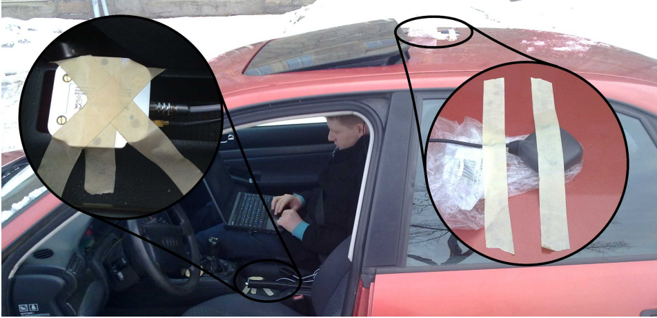
Figure 10.1: The mounting of the Xsens MTi-G in the car
