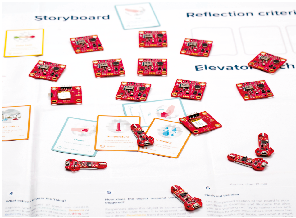
Figure 4.6: Electronic stickers employed by the users to prototype the smart objects.
