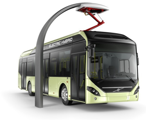
Figure 4.1: An electric bus using an inverted pantograph for charging.[76]
