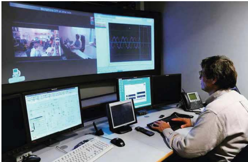
Figure 1.4: ABB-Shell collaboration room - an example of an integrated operations centre. The operator is located on-shore and has complete control of the off-shore facilities through visual tools. Courtesy ABB Strategic R&D for Oil, Gas and Petrochemicals.
