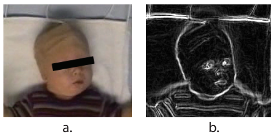
Figure 3.7: Shows the Sobel operator on a frame, highlighting good choices for creating FPs
