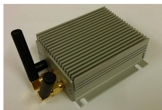
(b) USRP B200mini equipped with enclosure and antennas
