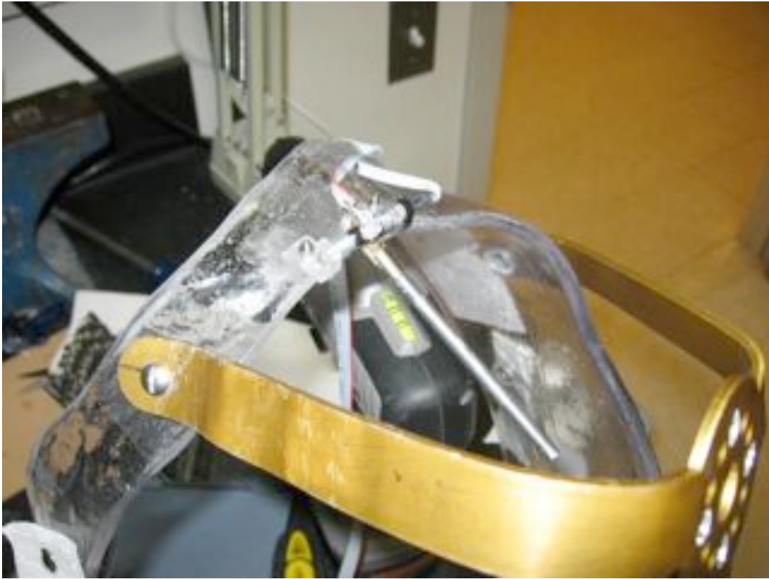
Figure 4.9 – Shoulder disarticulation amputee’s socket with a two-axis joystick for the evaluation of the vector projection algorithm
