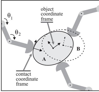
Figure 1: A typical dexterous manipulation problem: Moving an object from configuration  $A$  to configuration  $B$ .
