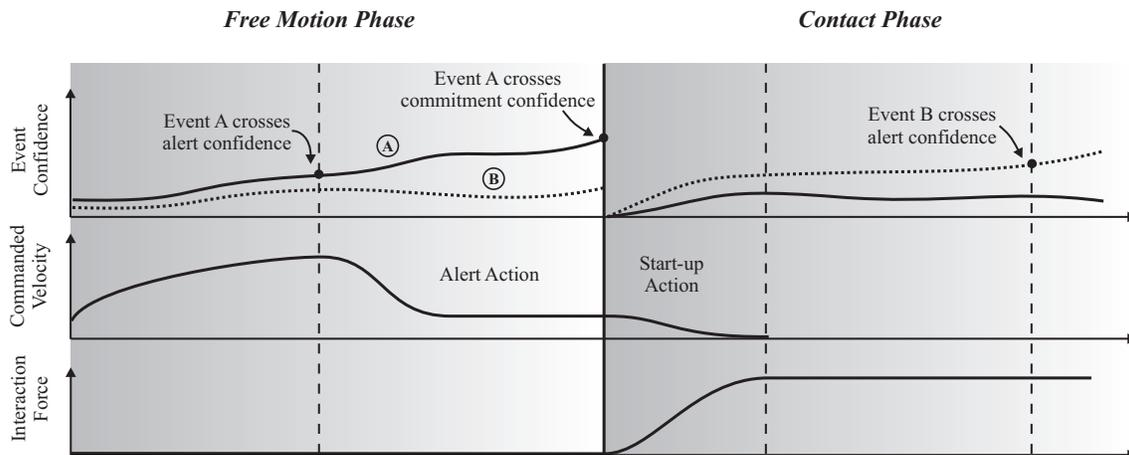
Figure 7: Events and transitions between phases (adapted from [13]).
