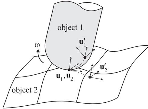
Figure 4: The contact frames for rolling.  $\mathbf{u}_1$  and  $\mathbf{u}_2$  are the contact frames for objects 1 and 2, respectively. After rolling occurs, the new contact frames will be  $\mathbf{u}'_1$  and  $\mathbf{u}'_2$ .
