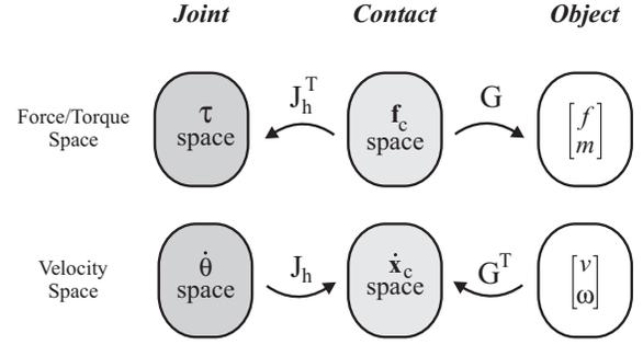
Figure 2: The role of the hand and grasp Jacobians. For the fingers,  $\tau$  is the vector of joint torques and  $\dot{\theta}$  is the vector of joint velocities. For the contacts,  $\mathbf{f}_c$  is the vector of contact forces and  $\dot{\mathbf{x}}_c$  is the vector of contact point velocities. For the object, the resultant force vector and the vector of object velocities are shown.
