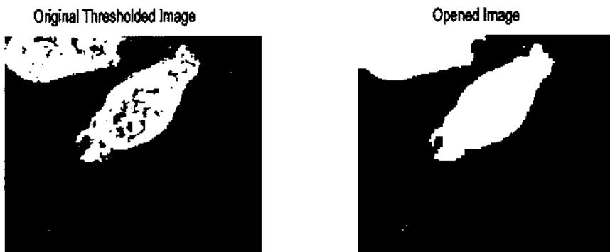
FIGURE 12.18 Application of the open operation to remove the dark patches in the binary cell image in Figure 12.15 (lower right). Using a 5 by 5 square structural element resulted in eliminating all of the dark patches.
