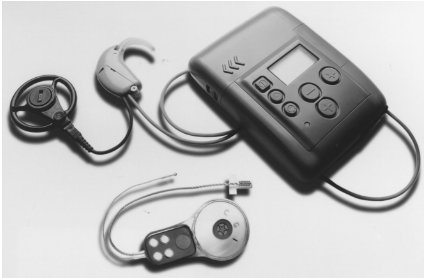
Figure 10.11 Auditory Brainstem Implant (Cochlear Corp.; Englewood, CO). The wearable speech processor (upper) has an ear-level microphone and associated transmitting antenna, and the magnet for attachment contains the batteries and sound processing circuitry. The implant portion (below) is comparable to a cochlear implant with a ball and ground electrode but with a flat surface array of electrodes at the end of the second cable that is placed on the medullary surface, over the cochlear nucleus. The implant also contains a receiving antenna, attaching magnet, and de-modulating circuit.
