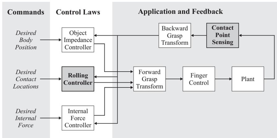
Figure 8: Control block diagram for manipulation with rolling.
