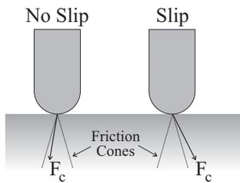
Figure 6: A representation of contact forces, with and without slip.
