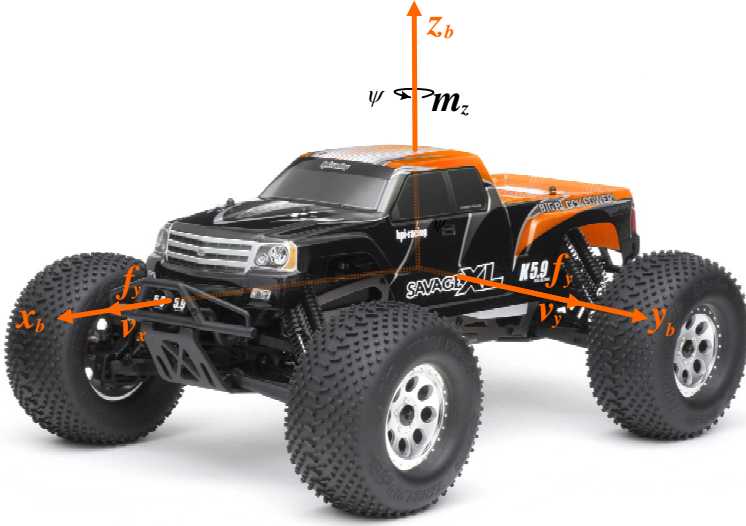
Figure 2.2: The force, moment and kinematic vectors in the xy -plane presented in the body frame.
