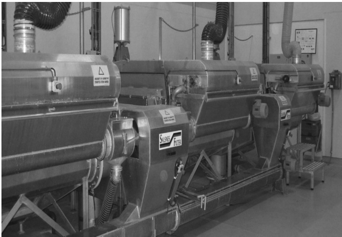
Figure 1.5 Tiendeholmen WWTP with three rotating belt sieves (Salsnes Filter SF6000) and 350 \mu\text{m} mesh size (Rusten & Ødegaard, 2006).
