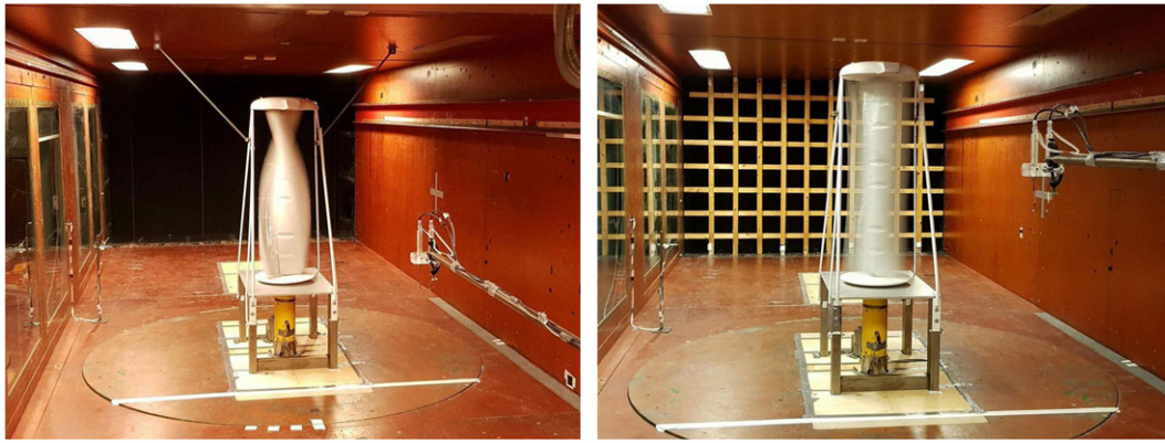
FIGURE 3 View of the setup inside the wind tunnel looking upstream. Left: Uniform inflow with additional support struts connecting the turbine to the ceiling. Right: Turbulent inflow with grid at the inlet of the test section [Colour figure can be viewed at wileyonlinelibrary.com ]
