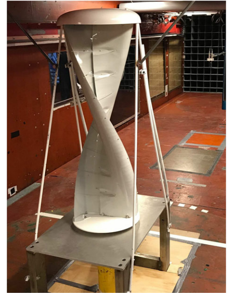
FIGURE 1 Savonius wind turbine used in the present experiment. Additional support struts connecting support structure to the ceiling are visible [Colour figure can be viewed at wileyonlinelibrary.com ]
