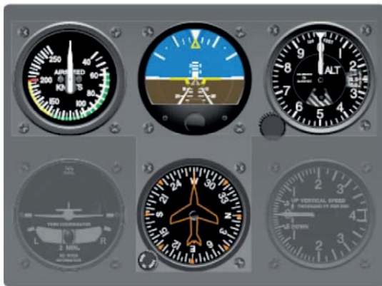
Figure 5. Basic T-arrangement (ASB, 2016).
