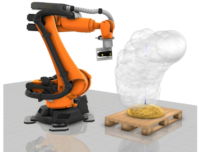
Fig. 2. Bounding spheres of the scanned point clouds are consecutively added to the robot simulation environment. Collisions with already scanned parts of the propeller blade can thus be avoided.
