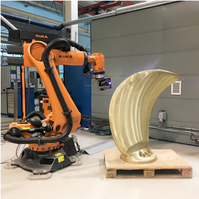
Fig. 1. An overview of the robotic scanning system setup including the robot manipulator with 3D camera and a highly skewed propeller blade.
