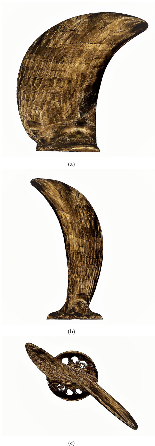
Fig. 5. The resulting combined point cloud of the propeller blade. The propeller blade is seen from the front (a), side (b), and above (c).
