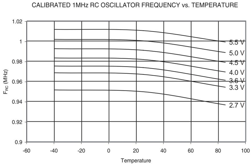
**Figure 193.** Calibrated 1 MHz RC Oscillator Frequency vs.  $V_{CC}$
