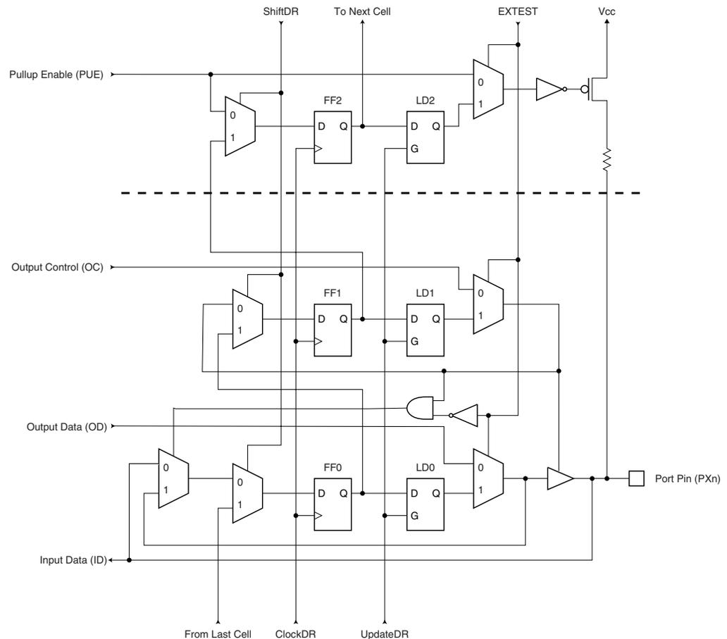
**Figure 125. General Port Pin Schematic diagram**
