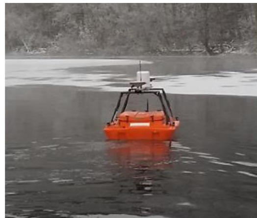
Figure 4.5: Sonar inspection of Storelva, Randselva and Begna (left, red), detail sonar inspection at the oxbow lakes in Ringerike (top right, dark blue) and Norbit - multibeam miniature boat (bottom right) (Høydal, 2017).
