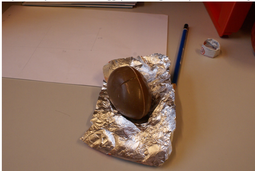
Figure 37: The result of a crashed thread that caused the fingers to continue closing in despite pressure threshold being surpassed.
