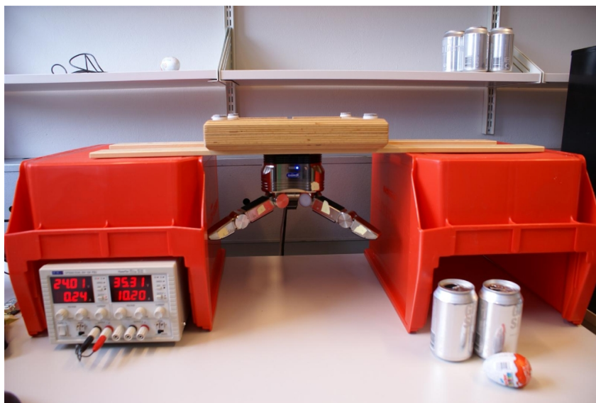
Figure 23: The testing setup for the gripping. The gripper is suspended in the air by supporting beams across two containers.
