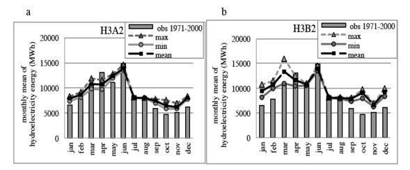
**Figure 11.** Range of monthly simulated hydropower energy under (**a**) A2 and (**b**) B2 emission scenarios in the 2070–2099 (far future).
