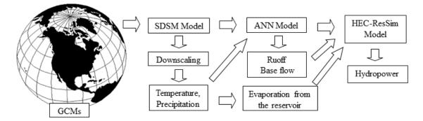
Figure 1. Methodology of climate change impact assessment on hydropower generation.
