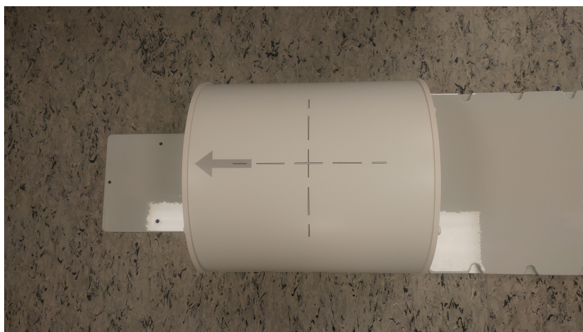
Figure 26: Image of the GRADE phantom placed on top of the flat MR overlay. The arrow symbol on the top of the phantom indicates which end of the phantom is inserted into the scanner first. The crosshair markings located next to the arrow is used to place the phantom, by aligning the cross with the laser cross produced by the laser bridge.
