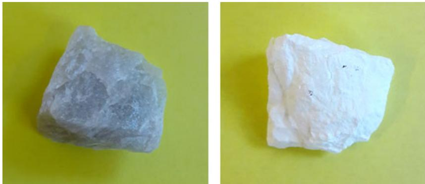
Figure 3: Sample A11 before (left) and after (right) heating to 1700 °C. The sample was held at 60 minutes at this temperature. The weight was 10.8 g, and the size of the samples are 2-3 cm.
