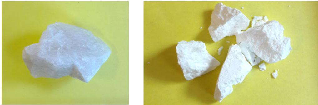
Figure 4: Sample P2 before (left) and after (right) heating. The sample was heated to 1600 °C and held for 120 minutes at this temperature. The weight of the sample was 9.7 g, and the size 2-3 cm.
