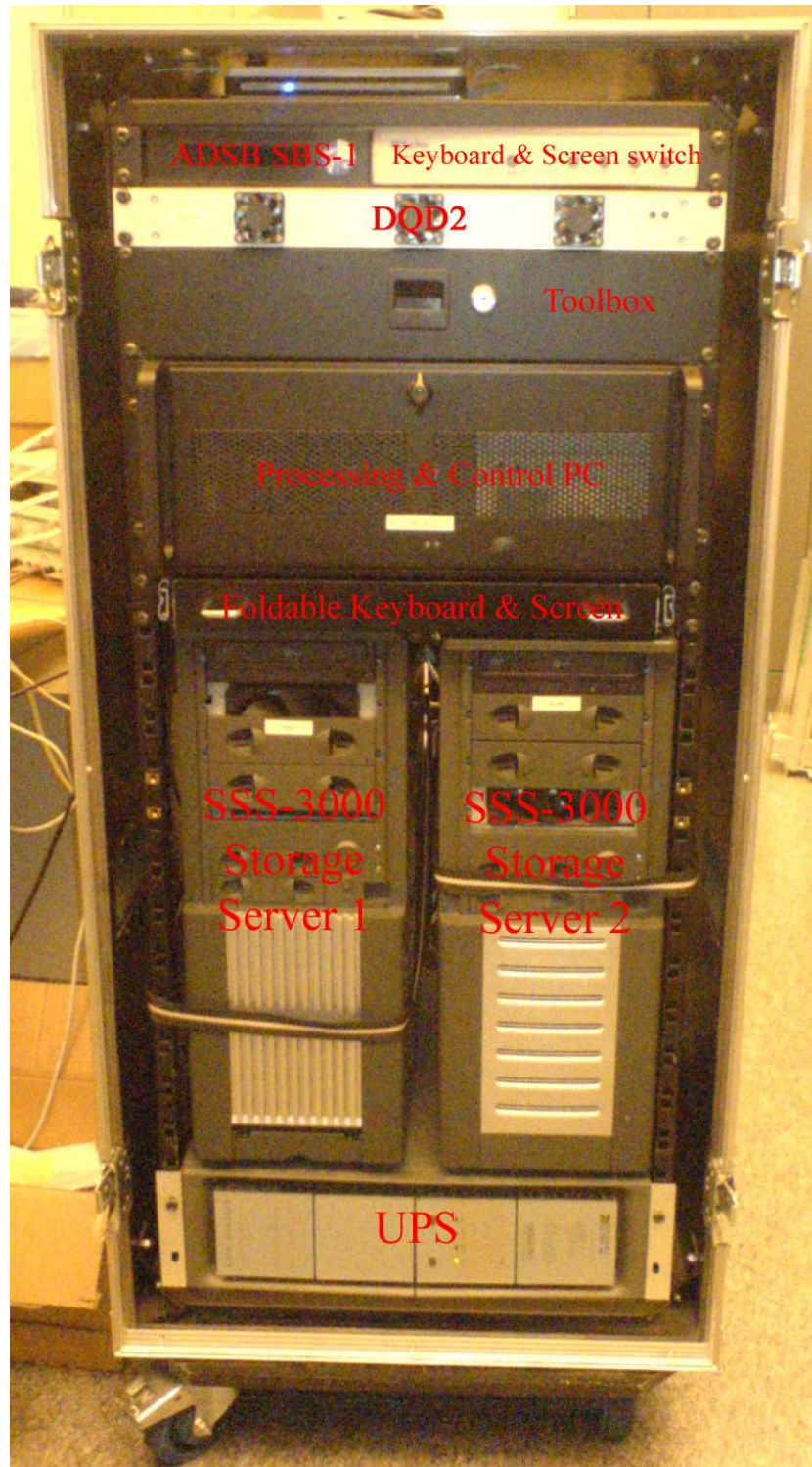
Figure 3.1: The hardware rack with the recording PC's, control PC and other hardware such as ADSB receiver and DQD2
