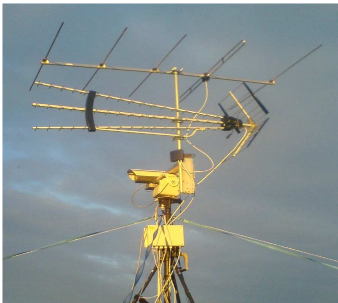
(a) Reference channel, FM radio antenna; TRIAX 5 element (upper antenna), DVB-T antenna; Televes DAT75 Digital Tv Aerial (lower antenna).
