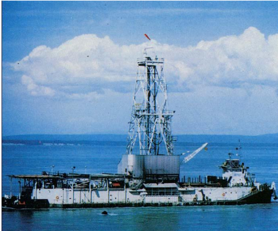
Figure 2.1: Cuss 1 , The first dynamically positioned vessel, equipped with four steerable thrusters. Courtesy of Friede & Goldman, LTD [5].
