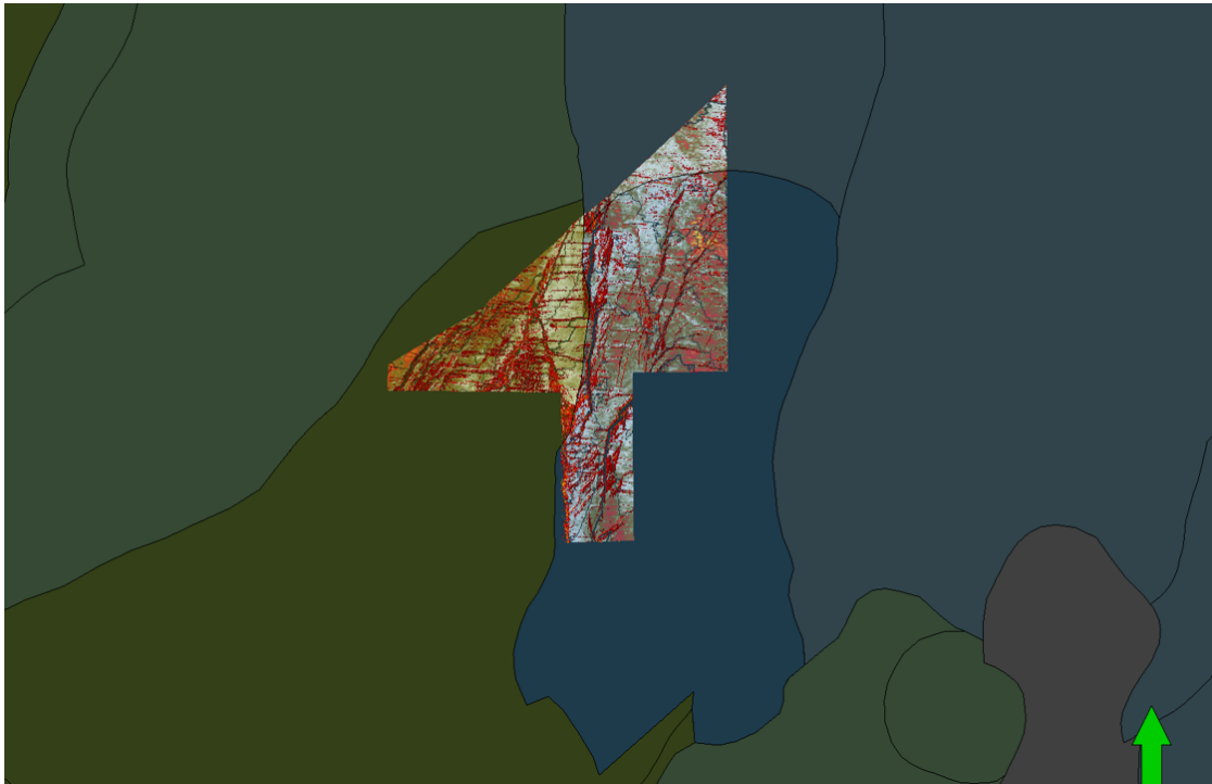
Figure 48: Favourability map for SEDEX-MVT suite deposits shown with surrounding the same features visualized as in the ROI delineation.
