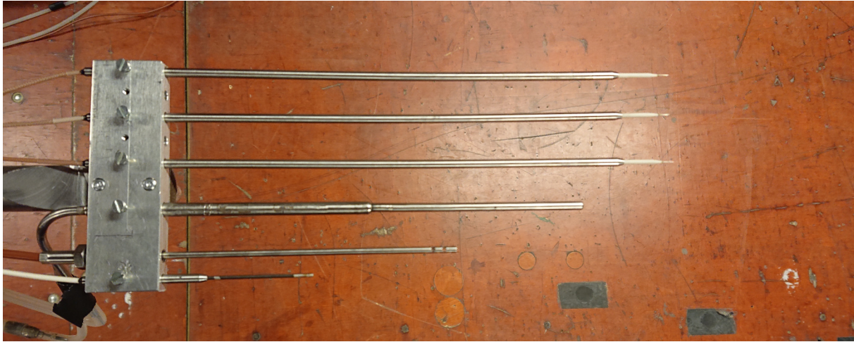
Figure 2.3: The probe holder seen from above. From the top: Hotwires 1, 2 and 3, the pitot-static tube, the T-type thermocouple and the RTD.
