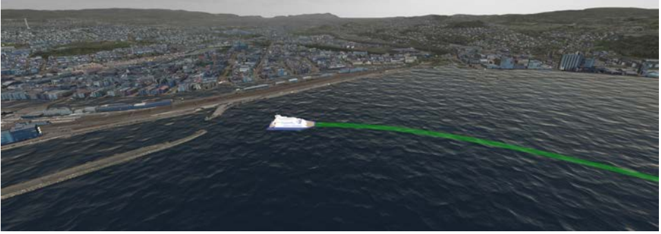
Figure 3.5: 3D-Visualization of a catamaran passenger boat in the Trondheim fjord using the Unity game engine Unity (2018), and the Hydroform Ocean System and Terraland plugins from the Unity Asset Store. The green arrow shows the predicted path of the vessel.
