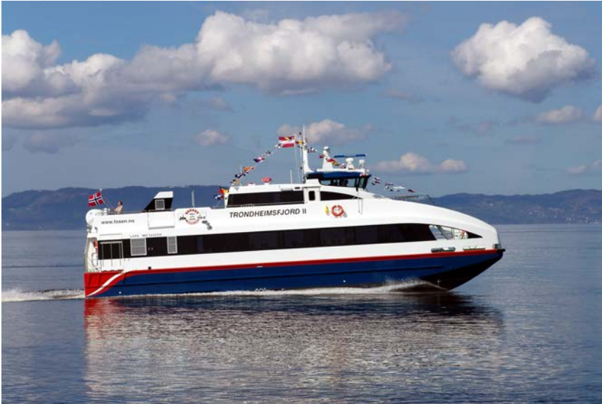
Figure 3.2: The MS Trondheimsfjord II is high-speed catamaran for passenger transport. Length 24.5 m, beam 8.0 m and maximum speed 16.5 m/s (32 knots). Reproduced with kind permission of Fosen Namsos Sjø ( http://www.fosennamsos.no ).
