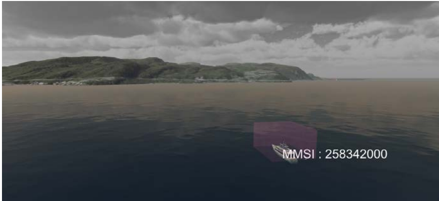
Figure 2.7: 3-D visualization of an AIS ship inscribed a rectangular prism. The color represent the risk collision index.
