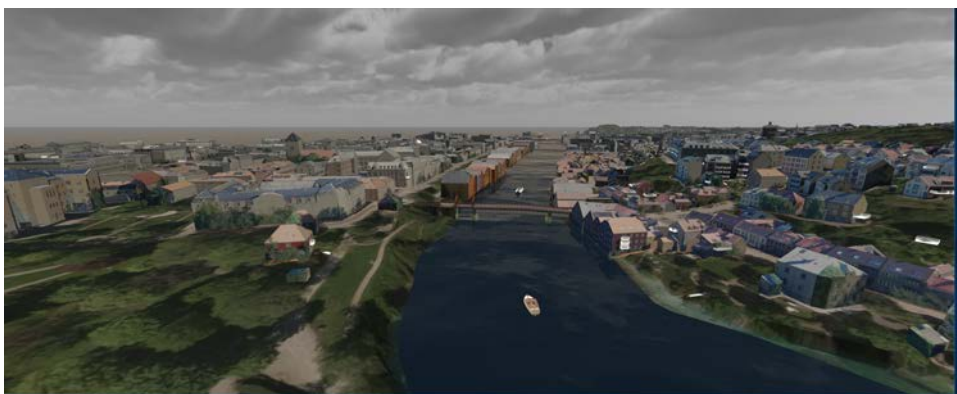
Figure 4.3: 3-D visualization of a pilot-controlled USV, which is moving up the Nidelven river in Trondheim. One live AIS ship is detected on the other side of the bridge.
