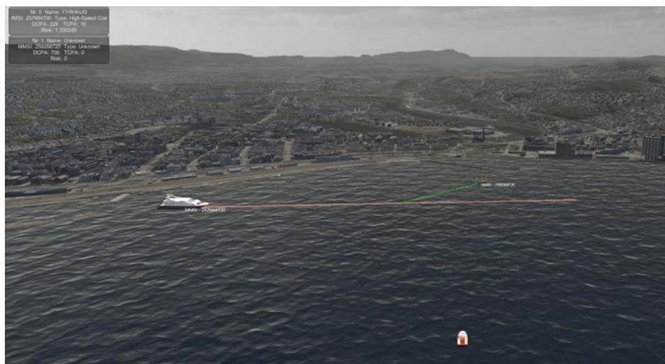
Figure 4.4: 3-D visualization of the pilot-controlled USV, which is approaching several live AIS ships outside the Trondheim harbor. The colored lines show the EKF predicted path of the approaching ships using AIS data. The collision risk index is computed online and a green line indicates small risk for collision, yellow is moderate risk, while a red line indicates high risk for collision.
