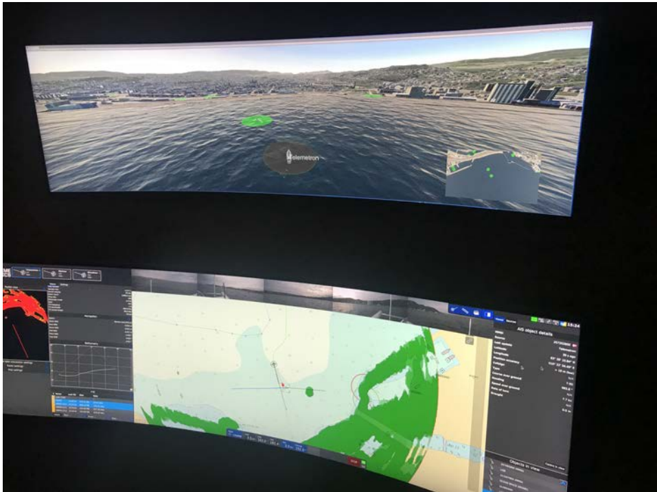
Figure 4.2: The vehicle control station for operation of a pilot-controlled USV in a mixed-reality environment. Unity is used to visualize the Trondheim fjord. The grey circle represents the safety region of the USV, while AIS detected ships are plotted with green, yellow or red circles to indicate if they present a collision risk or not for the USV. Reproduced with kind permission of Maritime Robotics AS.
