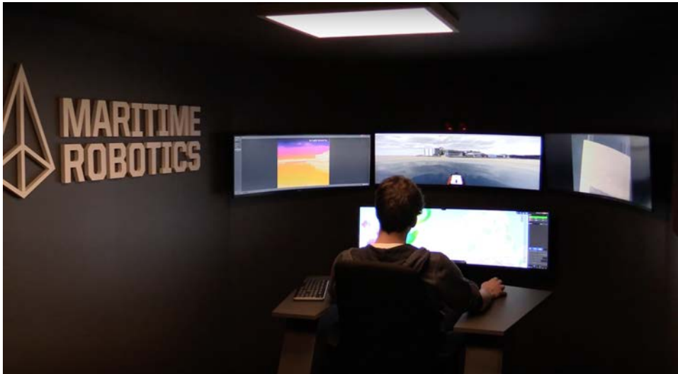
Figure 1.3: The Maritime Robotics AS vehicle control station (VCS) for 3-D visualization of ships in a mixed-reality environment.
