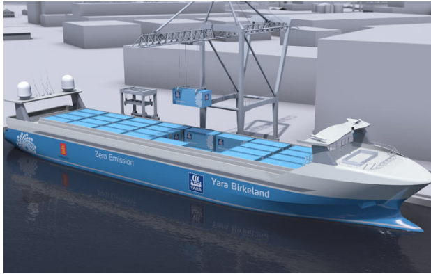
Figure 1.2: The Yara Birkeland, length 79.5 m, width 14.8 m and draught 6 m ( https://www.km.kongsberg.com ). Reproduced with kind permission of Kongsberg.
