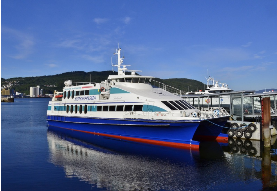
Figure 3.9: MS LADEJARL - Passenger ship (gross tonnage 490 t, length overall 38 m and breadth 10 m). Reproduced with kind permission of Fosens Namsos Sjø ( http://www.fosennamsos.no ).
