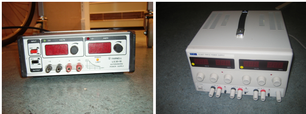
Figure 6.3: Power sources. Left: Farnell LS-30. Right: TTI EL302T.
