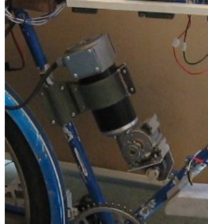
Figure 3.8: The propulsion motor; a Lenze Worm Geared motor
