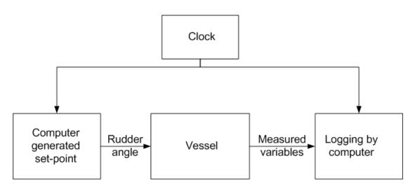
Figure 3.1: Set-up for system identification experiments
