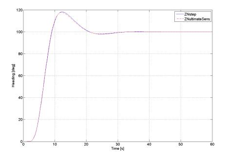
Figure 8.26: Step response using the ultimate-sensitivity and step-response parameters at 20 knots  $\,$
