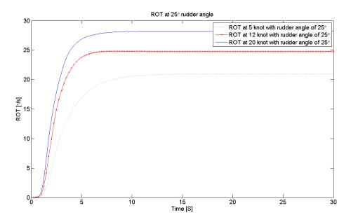
Figure 8.5: Model response at 5, 12 and 20 knots to a step in rudder angle of 25 degrees
