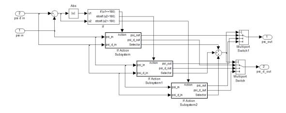
Figure 8.12: Upper level of the Simulink if block to choose the shortest direction
