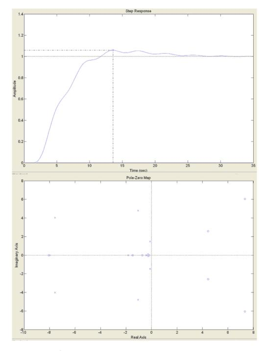
Figure 8.31: Pole / Zero plot and step response of the open loop with increased gains
