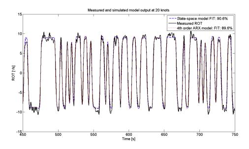
Figure 4.26: Model outputs at 20 knots
