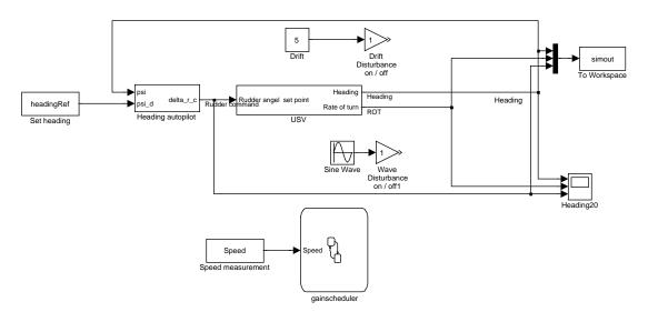
Figure 8.50: The complete Simulink model with state machine
