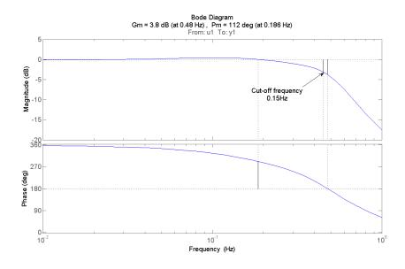
Figure 4.25: Bode plot for the  $4^{th}$  order ARX model at 12 knots
