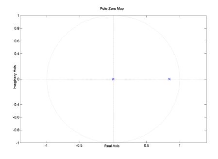
Figure 4.6: Pole-zero plot of the rudder pump model at 20 knots
