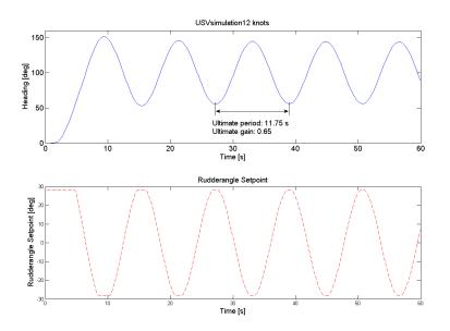
Figure C.26: Ultimate gain,  $K_u$  and period  $T_u$  of the Ziegler-Nichols ultimate-sensitivity method at 12 knots
