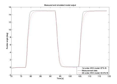
Figure C.9: Model output, 12 knots Rudder pump experiments
