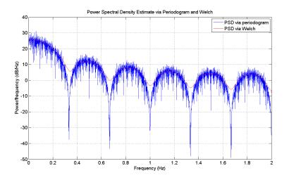
Figure 3.5: Frequency content of a PRBS input sequence updated at 0.33 Hz
