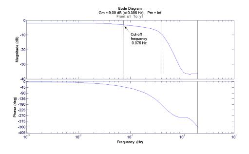
Figure 4.20: Bode plot for the 4th order ARX model at 5 knots
