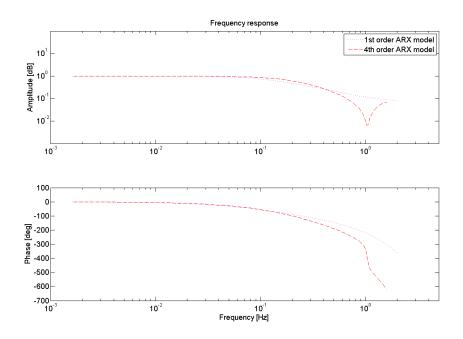
Figure C.10: Frequency response, 12 knots Rudder pump experiments
