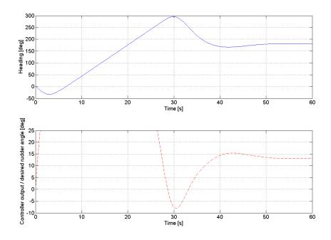
Figure 8.35: Integral windup for a step from zero to  $359^{\circ}$  at 20 knots
