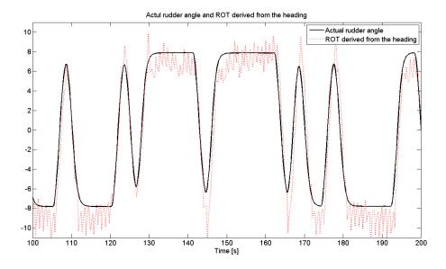
Figure 4.11: ROT derived from heading and actual rudder angle plotted together
