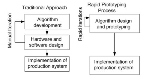
Figure 2.1: Traditional vs rapid prototyping design of a controller
