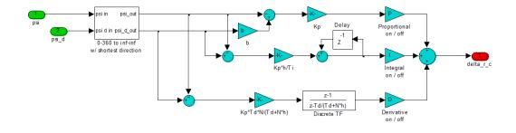
Figure 8.23: Simulink model of the controller
