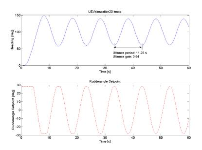
Figure C.27: Ultimate gain,  $K_u$  and period  $T_u$  of the Ziegler-Nichols ultimate-sensitivity method at 20 knots
