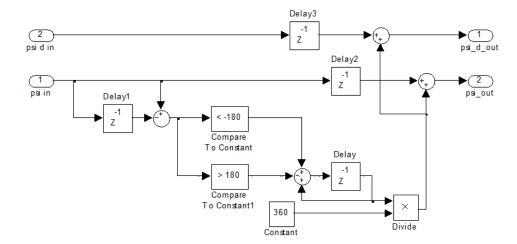
Figure 8.18: Simulink block removing the discontinuity in measurement and set point
