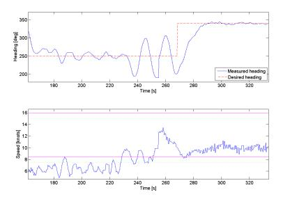
Figure 9.14: Gain scheduling with a step in desired heading
