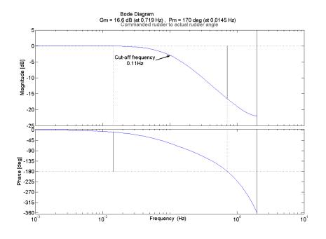
Figure C.6: Bode plot, 5 knots Rudder pump experiments
