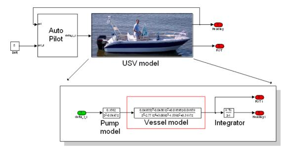
Figure 4.9: System identification of vessel dynamics
