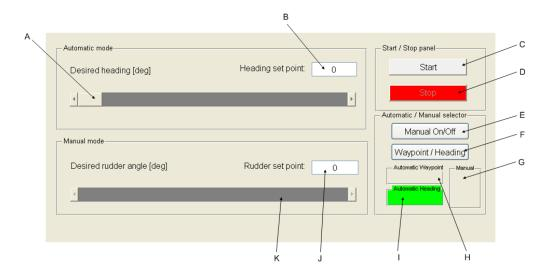
Figure 9.17: Graphical User Interface (GUI) for the autopilot
