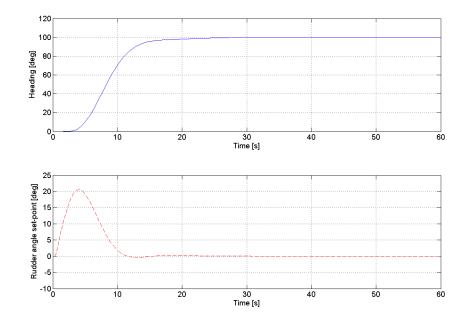
Figure 8.39: Controller performance at 5 knots
