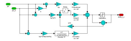
Figure 8.36: Simulink model of the controller with antiwindup
