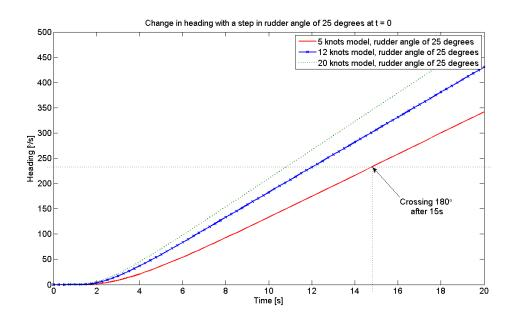
Figure 8.2: Heading response for 5, 12 and 20 knot models with a rudder angle of  $25^{\circ}$
