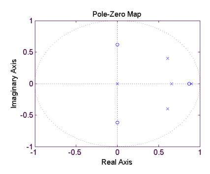
Figure 4.19: Poles and zeros of the 4th order ARX model at 5 knots
