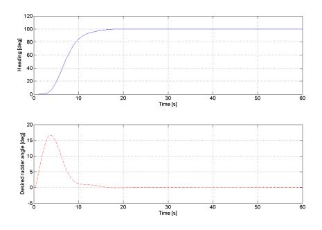
Figure 8.38: Controller performance at 20 knots
