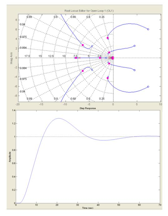
Figure 8.30: Pole / Zero plot and step response of the original Ziegler Nichols parameter
