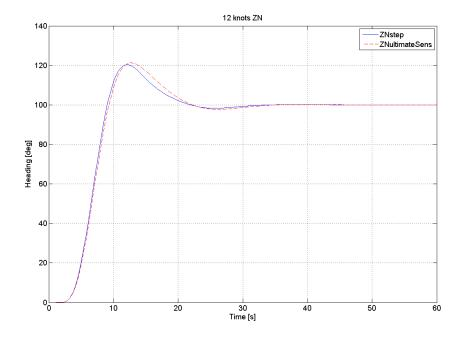
Figure C.29: ZN ultimate sensitivity vs. step-response at 12 knots
