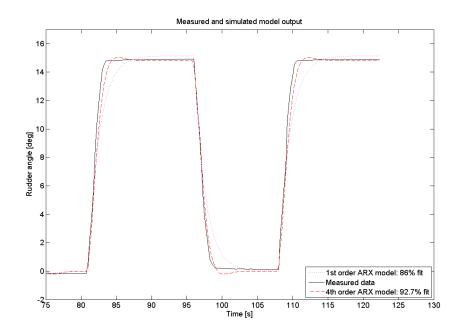
Figure C.2: Model output, 5 knots Rudder pump experiments
