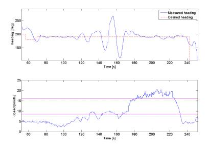
Figure 9.13: Gain scheduling with constant desired heading
