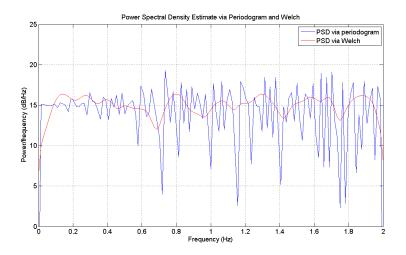
Figure 3.4: Frequency spectrum of a PRBS with period length 255 and sampled at 1 Hz
