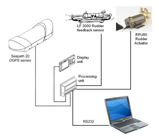
Figure 1.3: Measurment set-up
