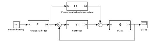
Figure 8.46: The set-point feed forward term in the block diagram
