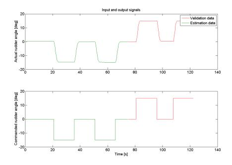
Figure C.1: Input/output data, 5 knots Rudder pump experiments
