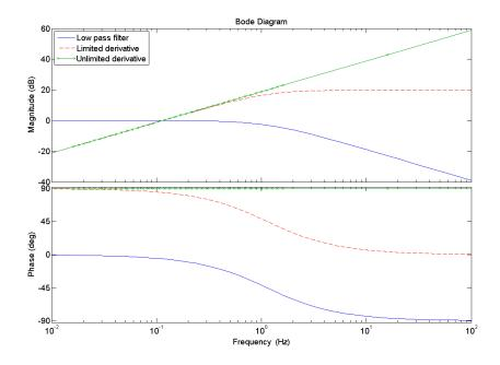
Figure 8.27: Bode plots of the unlimited and limited derivative action in addition to the low pass filter
