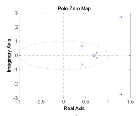
Figure 4.29: Poles and zeros of the  $4^{th}$  order ARX model at 20 knots
