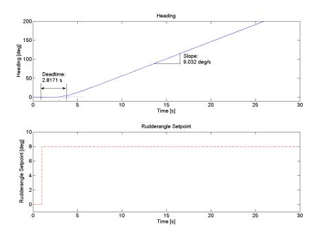
Figure 8.20: Slope R and deadtime  $L_d$  of the Ziegler-Nichols step response method at 20 knots
