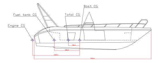
Figure 1.6: CAD drawing of the boat with CG, sideview
