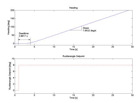
Figure C.23: Slope R and deadtime  $L_d$  of the Ziegler-Nichols step response method at 12 knots
