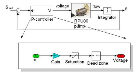
Figure 9.7: Actuator control loop with P controller)
