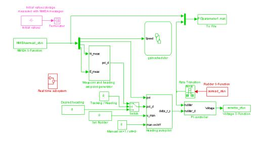
Figure 9.4: Sampling time in the MATLAB Simulink model; 0.05ms=red, 0.25ms=green, constant=magneta
