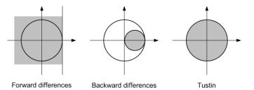
Figure 7.12: Mapping of the stability region in the s-plane to the z-plane, (Åström and Wittenmark, 1997)
