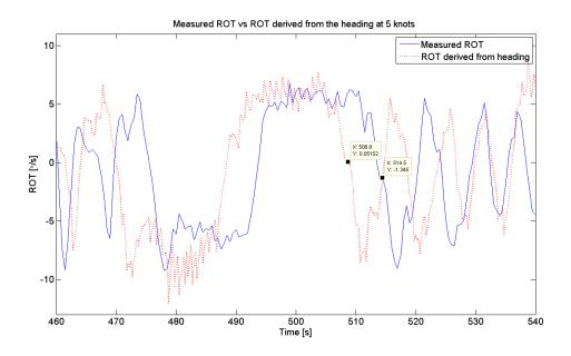
Figure 4.12: Measured and calculated ROT plotted together
