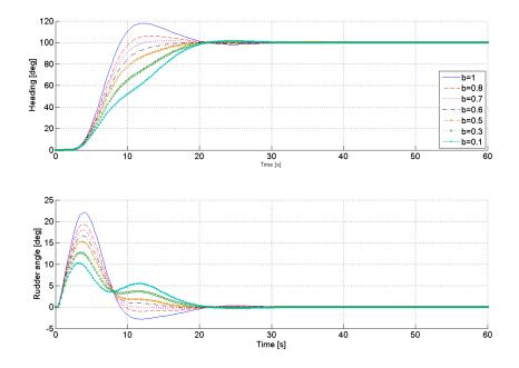
Figure 8.34: Different proportional set-point weighting for controller at 20 knots
