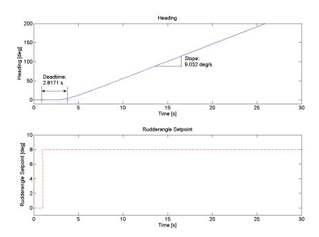
Figure C.24: Slope R and deadtime  $L_d$  of the Ziegler-Nichols step response method at 20 knots
