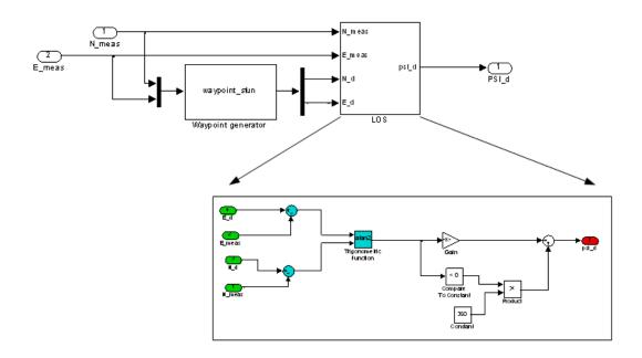
Figure 8.53: Way-Point Navigation block in Simulink
