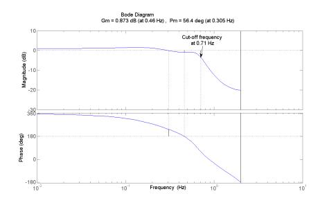
Figure 4.30: Bode plot of the  $4^{th}$  order ARX model at 20 knots
