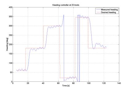
Figure 9.12: Implemented heading controller behaviour at 20 knots
