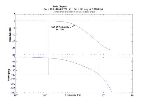
Figure C.13: Bode plot, 12 knots Rudder pump experiments
