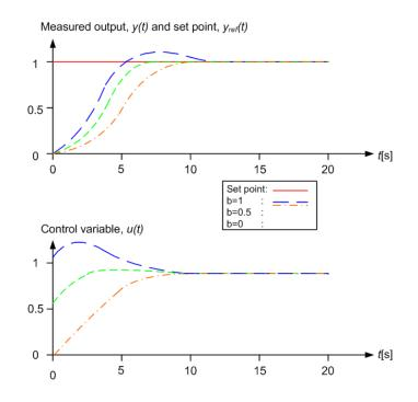
Figure 7.7: The usefulness of set point weighting, (Åström and Hägglund, 1996b)
