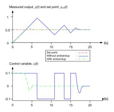
Figure 7.9: Effects of a PID controller with and without antiwindup, (Åström and Wittenmark, 1997)
