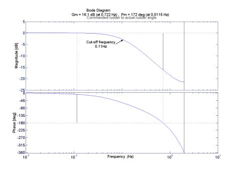
Figure 4.7: Bode plot of the rudder pump model at 20 knots
