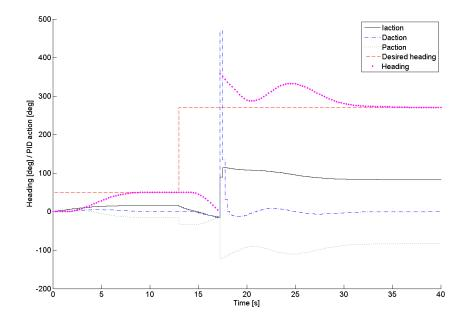
Figure 8.17: The effects of measurement discontinuity on a step from  $50^{\circ}$  to  $270^{\circ}$
