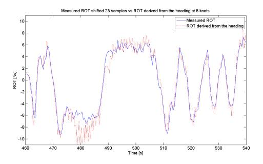
Figure 4.13: The measured ROT shifted 23 samples and plotted together ROT derived from the heading
