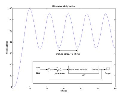
Figure 7.15: Ultimate gain,  $K_u$  and period,  $T_u$  of the Ziegler-Nichols ultimate-sensitivity method
