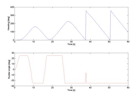
Figure 8.33: Unstable simulation on the "real model" with the controller parameters from root locus tuning without time delay
