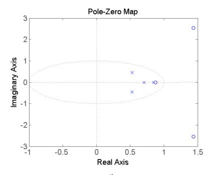
Figure 4.24: Poles and zeros for  $4^{th}$  order ARX model at 12 knots
