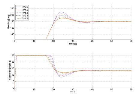
Figure 8.37: Antiwindup with different tracking times for a step from zero to  $359^\circ$  at 20 knots
