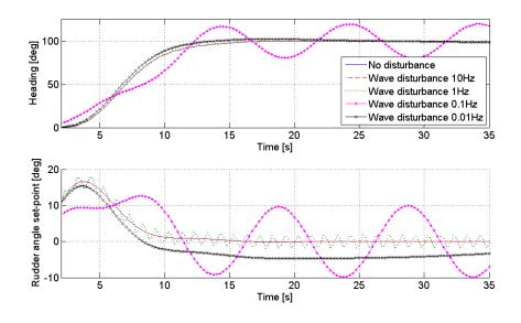
Figure 8.45: The effect of an oscillating disturbance in rate of turn
