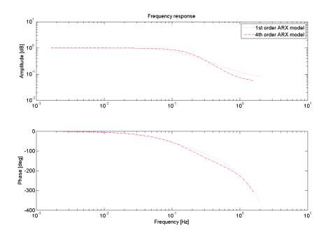
Figure C.17: Frequency response, 20 knots Rudder pump experiments
