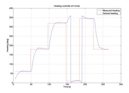
Figure 9.10: Implemented heading controller behaviour at 5 knots
