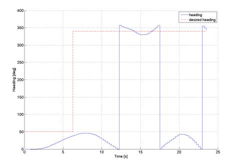
Figure 8.16: The effects of measurement discontinuity on a step from  $50^{\circ}$  to  $340^{\circ}$
