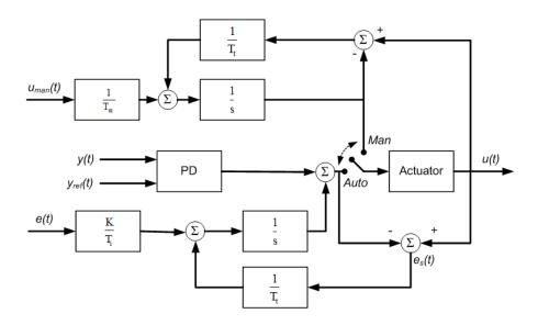
Figure 7.11: PID controller with bumpless switching between manual and automatic mode, (Åström and Wittenmark, 1997)
