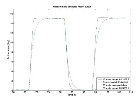
Figure 4.8: Model output of the rudder pump model at 20 knots with different speed models
