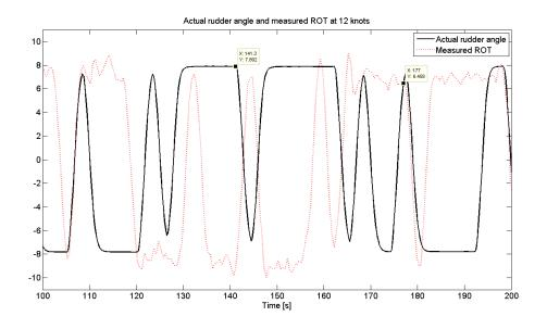
Figure 4.10: ROT and actual rudder angle plotted together
