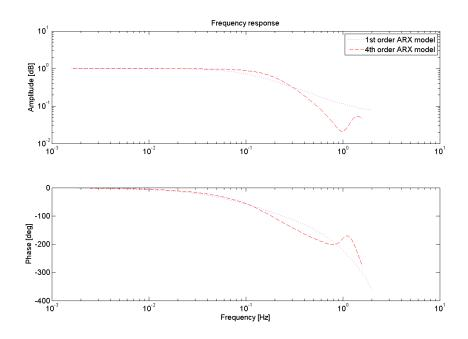
Figure C.3: Frequency response, 5 knots Rudder pump experiments
