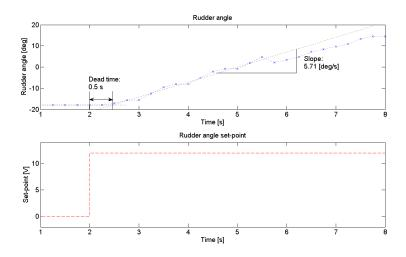
Figure 9.8: Step response for a step from -10.5 to  $10^{\circ}$ )
