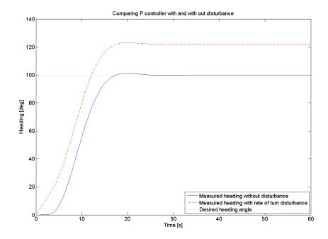
Figure 8.9: Steady state error with and without disturbance for a P controller
