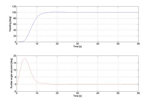
Figure 8.40: Controller performance at 12 knots
