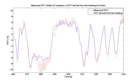
Figure B.3: Shifted ROT vs ROT derived from the heading at 5 knots
