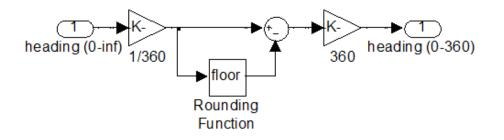
Figure 8.10: Discontinuous heading output  $(0-359^\circ)$
