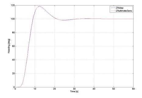
Figure C.30: ZN ultimate sensitivity vs. step-response at 20 knots
