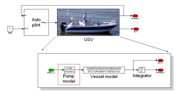
Figure 4.2: System identification of steering hydraulics
