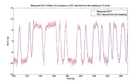
Figure B.6: Shifted ROT vs ROT derived from the heading at 12 knots
