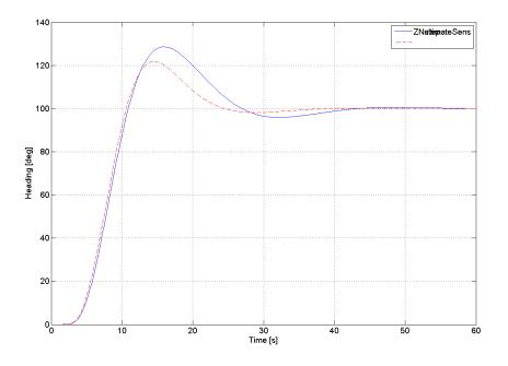
Figure C.28: ZN ultimate sensitivity vs. step-response at 5 knots
