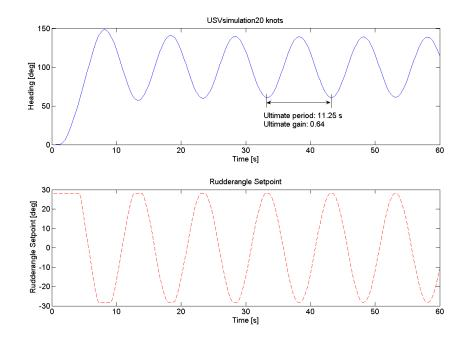
Figure 8.24: Ultimate gain,  $K_u$  and period  $T_u$  of the Ziegler-Nichols ultimate-sensitivity method at 20 knots
