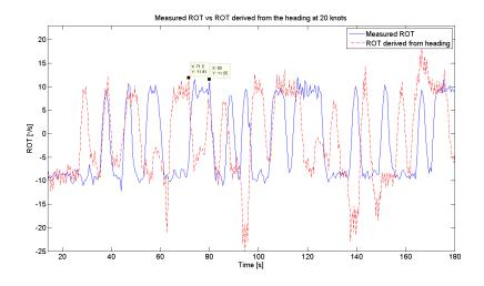
Figure B.8: Measured ROT vs ROT derived from the heading at 20 knots
