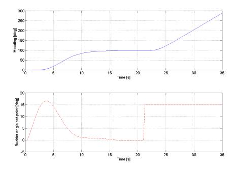
Figure 8.41: Transition from automatic to manual mode at 20 knots
