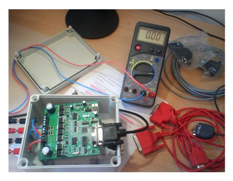
Figure 9.6: AX1500 I/O card from RoboteQ
