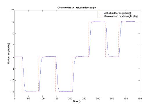
Figure 4.3: Rudder pump behaviour with Simrad P-controller
