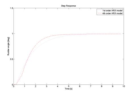
Figure C.11: Step response, 12 knots Rudder pump experiments
