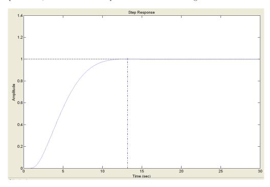
Figure 8.32: Step on a model with no time delay with root locus tuned parameters; Kp=0.5334, Ti=2.1, Td=0.96
