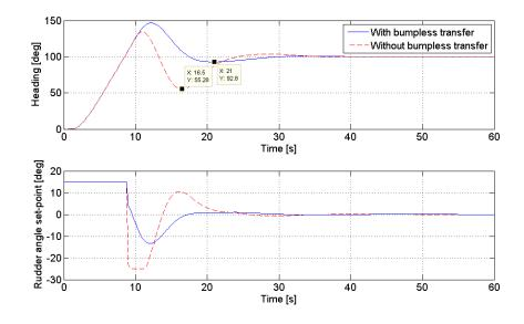
Figure 8.42: Transition from manual to automatic mode at 20 knots with and without bumpless transfer
