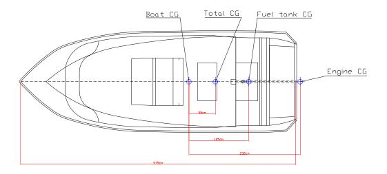
Figure 1.7: CAD drawing of the boat with CG, overview
