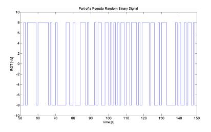
Figure 3.3: Part of a PRBS sequence with a length of 255
