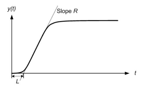
Figure 7.13: Slope R and deadtime  $L_d$  of the Ziegler-Nichols step response method
