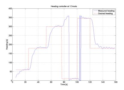
Figure 9.11: Implemented heading controller behaviour at 12 knots
