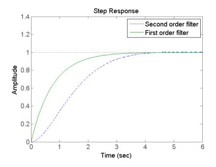
Figure 8.52: First order filter vs second order filter
