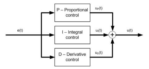
Figure 7.2: Parallel representation of the PID controller
