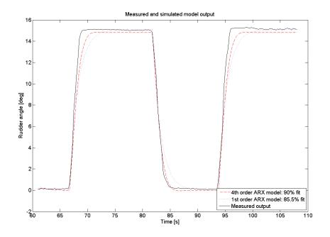
Figure 4.5: Rudder pump model output at 20 knots
