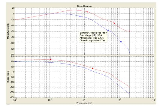
Figure 8.49: Bode plot of the input sensitivity and the closed loop with proportional set-point weighting
