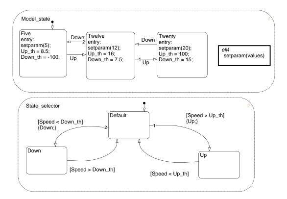
Figure 8.51: State machine for the gain scheduling algoritm
