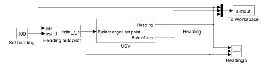
Figure 8.22: Simulink model of the USV simulation
