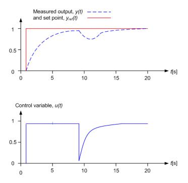
Figure 7.10: A system switching from manual to automatic mode without bumpless transfer, (Graebe and Ahlén, 1996)
