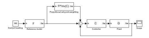
Figure 8.47: Feed forward term is multiplied by the inverse of the controller
