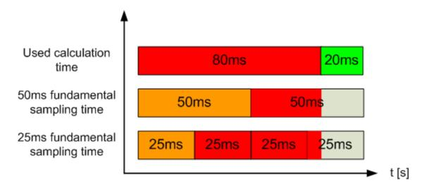
Figure 9.5: The two different fundamental sampling times with a calculation time of  $80\mathrm{ms}$
