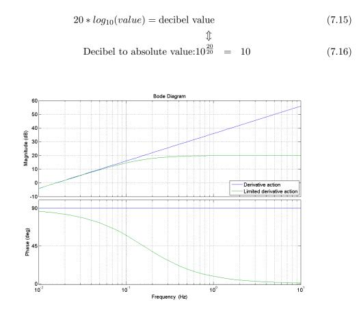
Figure 7.6: Bode plot of the unlimited and limited derivative action
