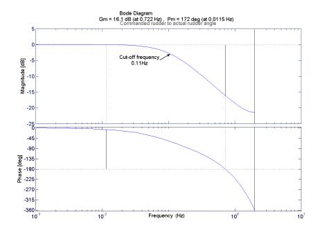
Figure C.20: Bode plot, 20 knots Rudder pump experiments
