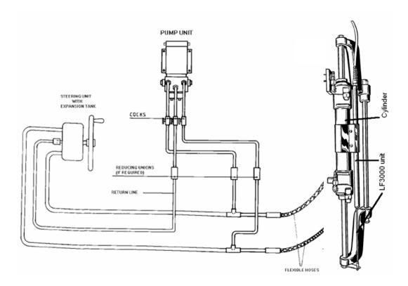
Figure 1.5: Hydraulic steering system, (www.simradyachting.com)
