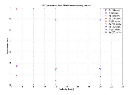
Figure 8.25: Kp, Ti and Td parameters for all speeds derived from ZN ultimate sensitivity
