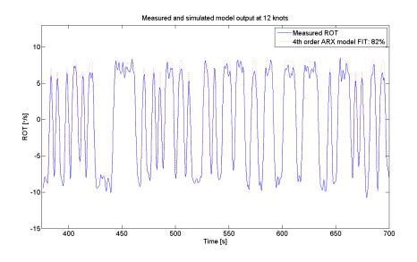
Figure 4.23:  $4^{th}$  order ARX model output vs measured ROT at 12 knots
