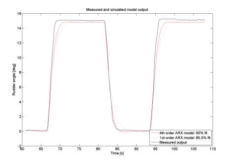
Figure C.16: Model output, 20 knots Rudder pump experiments
