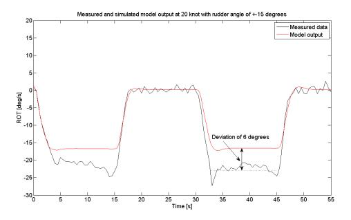
Figure 5.1: Deviation between measured ROT and model predicted ROT at  $15^{\circ}$  rudder angle
