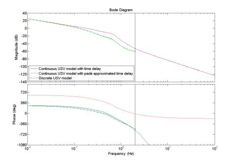
Figure 8.28: Bode plot of the model transfer functions in discrete/continuous time with/without Padé approximation
