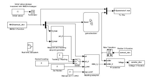
Figure 9.1: The MATLAB Simulink model for the implementation
