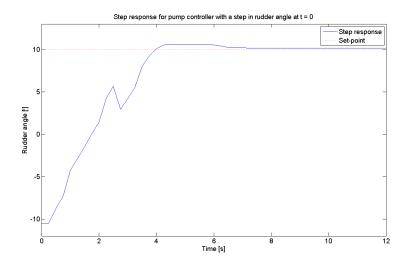
Figure 9.9: Step response for a step from -10.5 to  $10^{\circ}$ )
