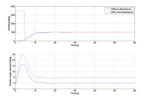
Figure 8.44: The effect of a constant disturbance in rate of turn
