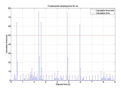
Figure 9.3: Calculation time with 50 ms fundamental sampling time
