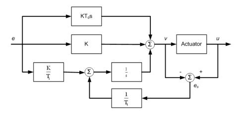
Figure 7.8: A PID controller with tracking antiwindup, (Åström and Wittenmark, 1997)
