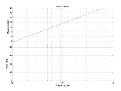
Figure 7.5:  $90^{\circ}$  phase lead of the derivative action
