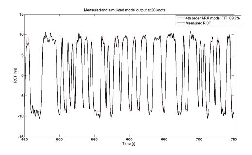
Figure 4.28:  $4^{th}$  order ARX model output vs measured ROT at 20 knots
