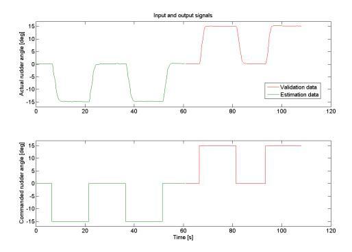
Figure 4.4: Rudder pump range for estimation and validation at 20 knots
