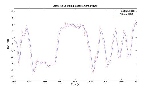
Figure 4.14: Filtered and unfiltered ROT
