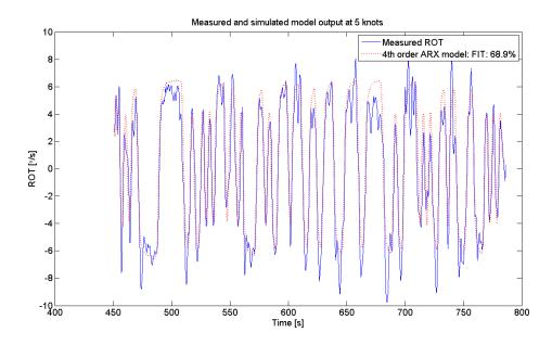
Figure 4.18: Model output of 4th order ARX model at 5 knots
