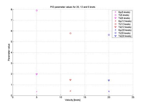
Figure 8.21: Kp, Ti and Td parameters for all speeds derived from ZN step response
