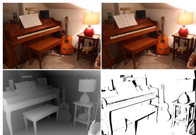
FIGURE 18. “Piano” stereo pair. From left to right: left and right views (top), disparity map with holes filling of the right view and occlusion map of the right view. Occluded regions appear in black.
