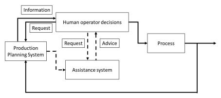
Fig. 1. Human-machine interface for decision making [15].
