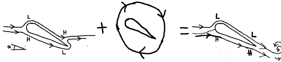
Figure 3.2: Kutta-Zhukovsky explanation of the generation of lift by adding large scale circulation to potential flow
