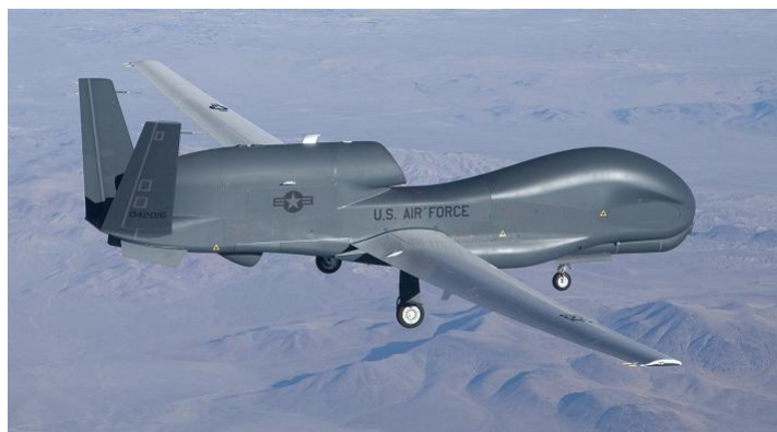
Figure 1.1: The RQ-4 Global Hawk is an unmanned US surveillance aircraft designed to operate autonomously. (Image courtesy of Northrop Grumman [25])
