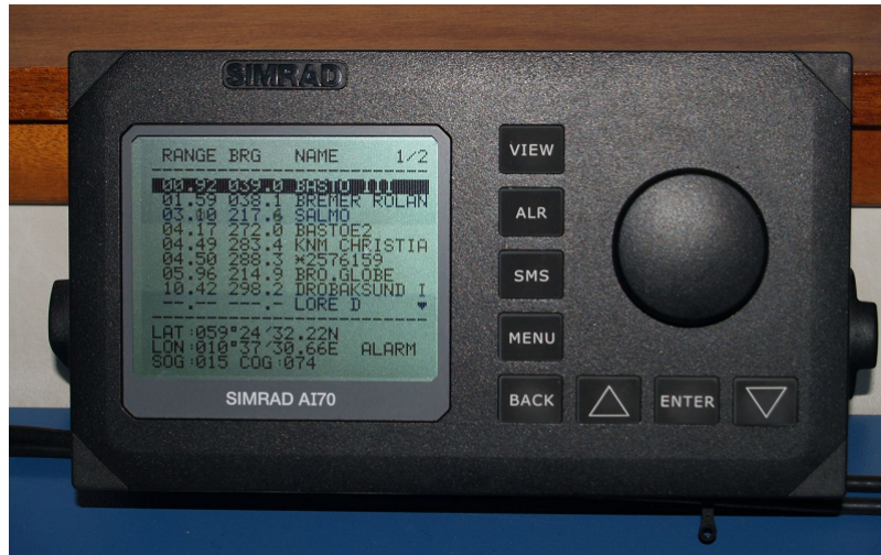
Figure 5.3: A text-only AIS display, listing nearby vessels with range, bearing and name.
