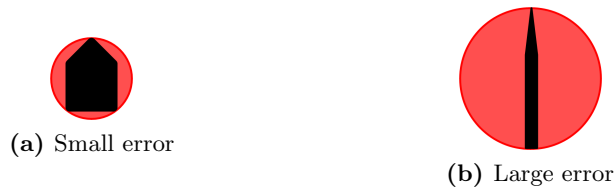
Figure 3.3: The error in the C-space approximation depends on the length-to-breadth ratio of the vessel. For the vessel in (a), the circle approximation is good, resulting in a small error. For the vessel in (b), the error is quite large as shown by the size of the red area.
