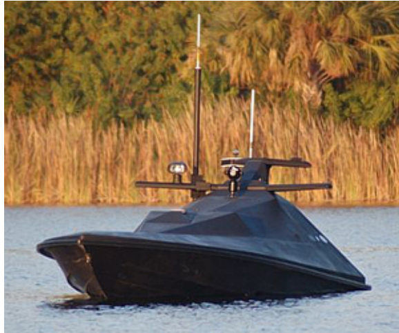
Figure 1.2: The Interceptor is an unmanned surface vessel (USV). Commanded by an on-board computer it is designed to autonomously complete the goals it is given by an operator [49]. Applications for USVs include patrol and surveillance, for instance for harbour security and customs, mapping of the seabed, geological surveys, etc. (Image courtesy of 5G Marine Systems [6])
