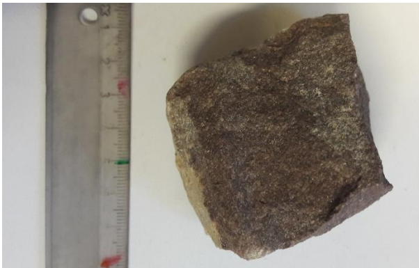
Figure 5: A sample of quartz type D, prior to heating. The sample weighs approximately 200 g.
