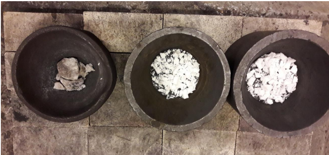
Figure 9: Three different quartz samples after shock heating at 1500 °C. Quartz type D, A and B shown from left to right.
