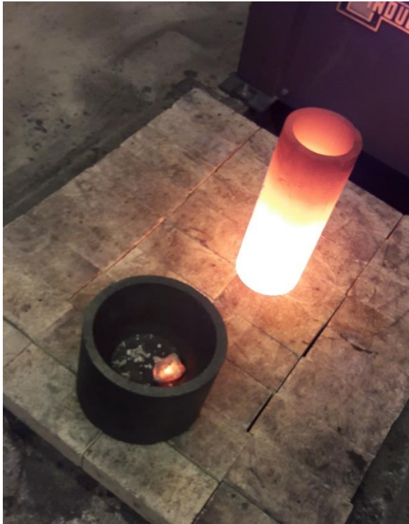
Figure 6: A quartz sample seconds after being poured from the warm crucible in the back at 1500 °C to the crucible in front at room temperature. The quartz is still glowing.
