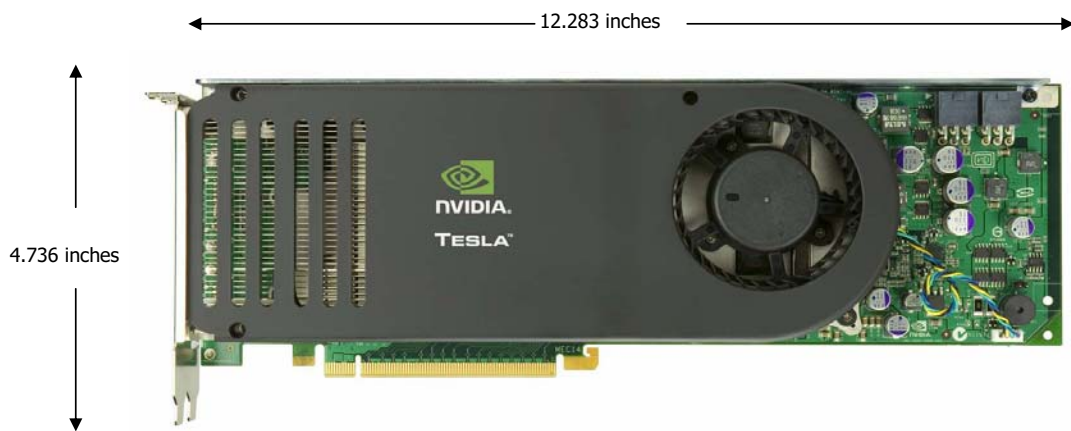
Figure A.1: Dimensions of the C870 board.
