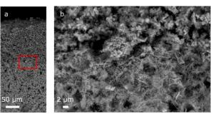
Figure 9. SEM micrographs of CaSi exp. 2 fracture surface.
