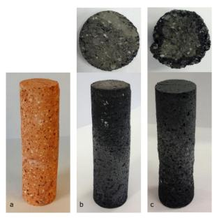
Figure 3. Macroscopic observations of pristine Moler (pre-exp. 1) in a), exp. 1 sample with a fracture cross section in b), and exp. 2 sample with a fracture cross section in c). Note the visible, glassy outer Rx-layer in the cross sections.
