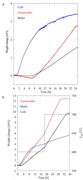
**Figure 2.** Weight change of the three materials as function of time during exposure to Na. a) exp. 1, b) exp. 2, where  $T_{Na}$  given by dotted line showing  $T_{Na}$  changed from 600 °C to 700 °C at ~18 h. In both a) and b), the materials are listed from highest to lowest total weight change at the end of the test.
