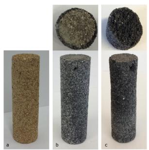
Figure 5. Macroscopic observations of pristine vermiculite in a), exp. 1 sample with a fracture cross section in b), and exp. 2 sample with a fracture cross section in c). In b), note the visible outer Rx-layer in the cross section as well as the inner core with similar appearance as the pristine material.
