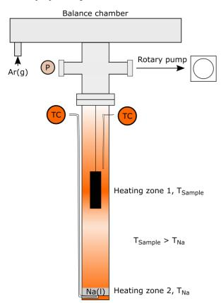
Figure 1. Schematic of the experimental thermogravimetric analysis setup (not to scale).
