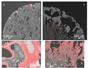
Figure 4. SEM micrographs of the polished cross sections of the Moler samples a)-b) exp. 1, and c)-d) exp. 2. Red area in b) and d) from EDS Na mapping.
