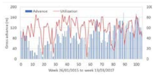
Figure 10. Weekly utilization and gross advance rate (based on data from Suescún and Jiménez, 2017).
