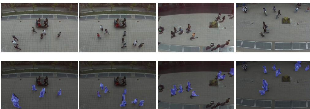
Figure 6: Results of proposed GKIM on UCD dataset. The detection and localization of anomalous entities are overlaid on the original frames and annotated in blue for the purpose of visualization. The pedestrian flows representing deviations from what have been observed before are detected accurately by GKIM in all the four scenes.
