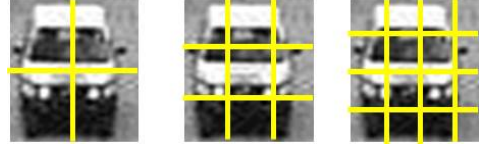
Figure 3: Multiple gridding. A frame patch is decomposed into three-level gridding that is 2x2, 3x3, and 4x4, where each grid is a block. The Multiple-level gridding captures information at different granularities.
