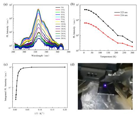
**Figure 5.** The photoluminescence properties and electroluminescence of AlGaN nanorod LEDs: (**a**) The spectra of temperature dependent PL; (**b**) the temperature dependence of PL intensity of peaks at 325 and 334 nm; (**c**) the temperature dependence of normalized integrated PL intensity of the AlGaN nanorod LEDs; and (**d**) optical image of the violet electroluminescence from the AlGaN nanorod LEDs.
