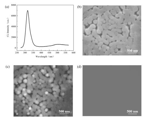
**Figure 6.** The cathodoluminescence properties of AlGaN nanorod LEDs: (**a**) The CL spectrum at room temperature; (**b**) the SEM image of CL mapping; (**c**) the CL mapping image at the wavelength of 318 nm; and (**d**) the CL mapping image at the wavelength of 500 nm.
