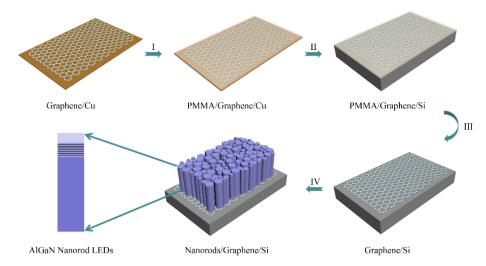
**Figure 1.** Schematic diagram of the key processes involved in the graphene transfer procedure and the metal organic chemical vapor deposition (MOCVD) growth of AlGaN nanorod LEDs: (I) Spin-coated poly(methyl methacrylate) (PMMA) onto graphene on Cu foil; (II) transfer of graphene with PMMA onto Si substrate; (III) dissolving PMMA; and (IV) MOCVD growth of AlGaN nanorod light emitting diodes (LEDs).
