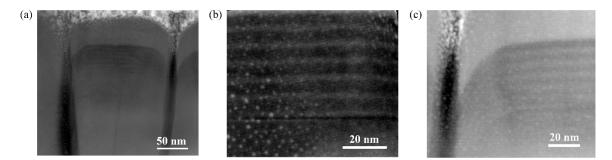
**Figure 3.** The structure of AlGaN nanorod LEDs: (**a**) cross-sectional STEM image of a single AlGaN nanorod LED; (**b**) the amplified MQWs structure; and (**c**) the curved downward MQWs and p-AlGaN.
