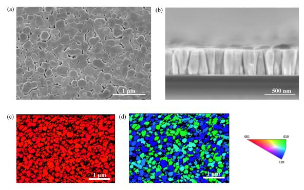
**Figure 2.** The morphology and orientation of AlGaN nanorod LEDs: (**a**) The 25° tilted-view SEM image of AlGaN nanorod LEDs; (**b**) the cross-sectional SEM image of AlGaN nanorod LEDs; (**c**) the normal-direction electron backscatter diffraction (EBSD) inverse pole figure (IPF) image of AlGaN nanorod LEDs; (**d**) the transverse-direction EBSD IPF image of AlGaN nanorod LEDs.
